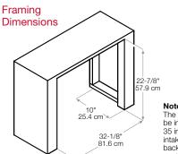
The fireplace needs to be installed to ensure 35 in<sup>2</sup> (226 cm<sup>2</sup>) of intake air, into the back of the unit, on a continuous basis.
