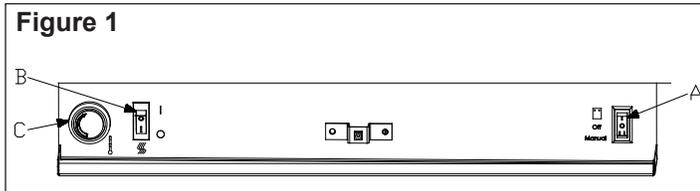
To access the controls, swing down the front cover panel located on the lower front of the fireplace. (Figure 1)
