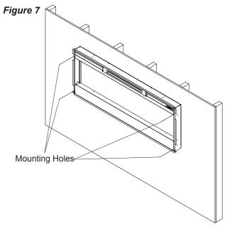
inner casing on the left and right hand side. There are 2 screws per side, upper and lower going into a stud. (Figure 8)
