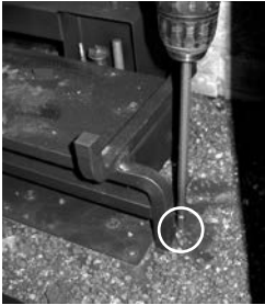
Diagram 1: Remove the left and right screws.
