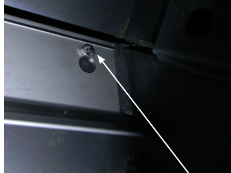
Ensure deflector is seated so bolts are situated at the top of the keyhole before tightening.
