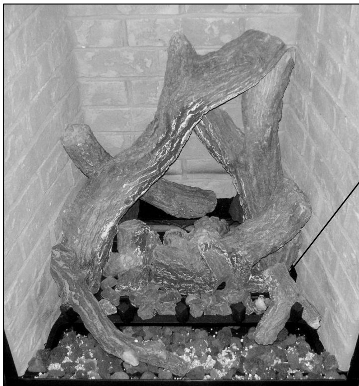
Step 6: Add lava rock to the bottom of the burner pan. Add glowing embers to the top of the ember plates and front burner tube. And sprinkle vermiculite over the lava rock. Do not place any media within Pilot Shield Area (see above).
