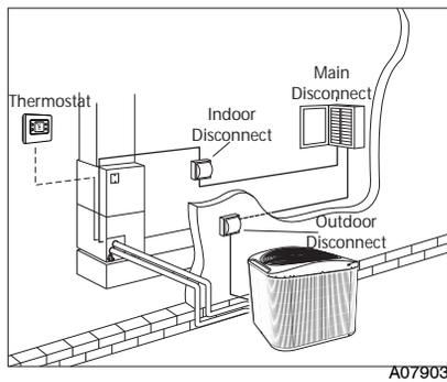
Fig. 1 - Electrical Disconnects
