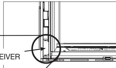
If receiver removal is necessary, remove the left access panel from the front of the appliance. Remove the 2 screws holding the receiver in place. Pull the receiver through the access hole and replace.
