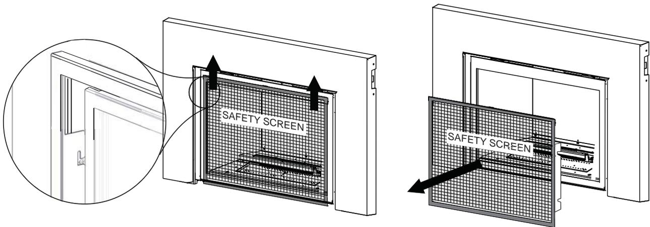
The optional front must be removed to allow the door to be opened or closed. Release the top left and right door latches, located at the top of the door. Tilt forward and lift from slots.
