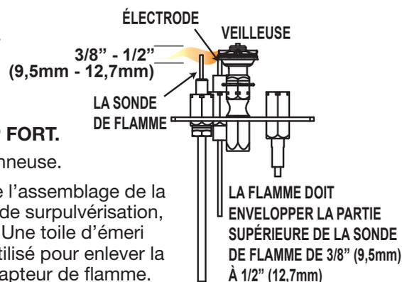
LA FLAMME DOIT ENVELOPPER LA PARTIE SUPÉRIEURE DE LA SONDE DE FLAMME DE 3/8" (9,5mm) À 1/2" (12,7mm)
