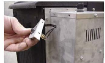
Because the blower is thermally activated, when turned on, it will automatically start approximately 15-30 minutes after lighting the appliance and will run for approximately 30-45 minutes after the appliance has been turned off. Use of the fan increases the output of heat.
