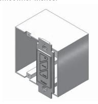
Locate and secure magnet plate using 2 'long' screws provided
