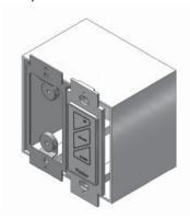
10. Place and secure cover plate to box using 4 screws provided
