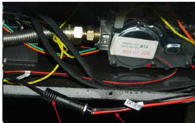
DC supply wire from wiring harness
