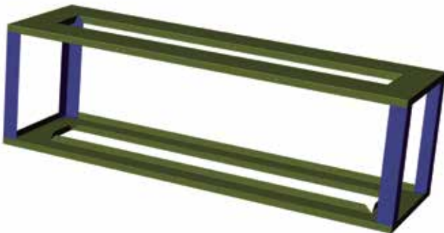
Diagram 3 - Corner supports with top frame
