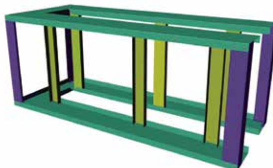
Diagram 5 - Install Inside vertical supports
