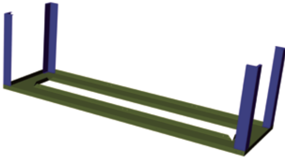
Diagram 1 - Corner supports on lower frame.
