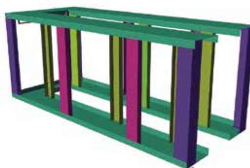
Diagram 7- Install outside vertical supports (B1) with 4 screws each
