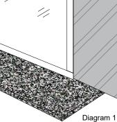
**Note:** All non-combustible and combustible facing material should butt up cleanly to the flanges around the firebox opening.
