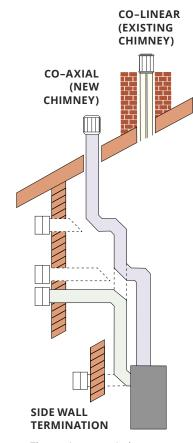
The maximum vertical vent run on a Horizon/H4 can not exceed 40 feet in total length. The engine can be either top or rear vented.
