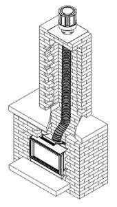
Natural Gas RF24JDN-CA Propane RF24JDP-CA Colinear New with AutoFire 2x3" Flex vent
