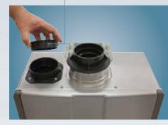
For PVC/CPVC/PP configurations, the intake cap is removed and discarded. With this option, installers can use 3- or 4-inch PVC/CPVC/PP pipe for the intake and exhaust.
