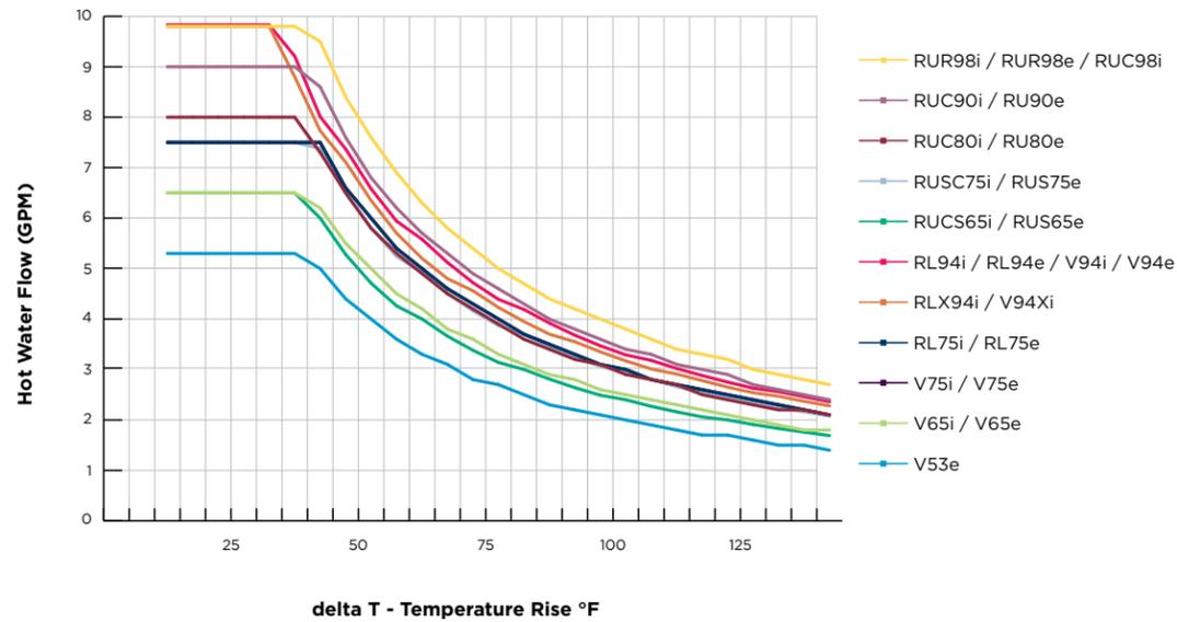
Tankless water heater output is based on Delta T, which is the difference between the incoming water temperature and the requested output temperature. This chart is used along with other factors to help size the Rinnai tankless model for your application.
