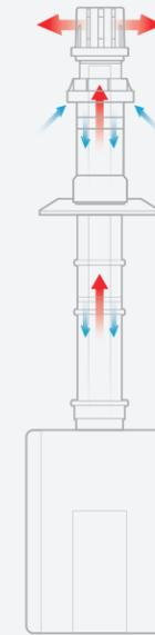
Venting available in vertical and horizontal configurations. Concentric structure allows hot exhaust to exit through interior tube, while fresh air enters through the outer layer.
