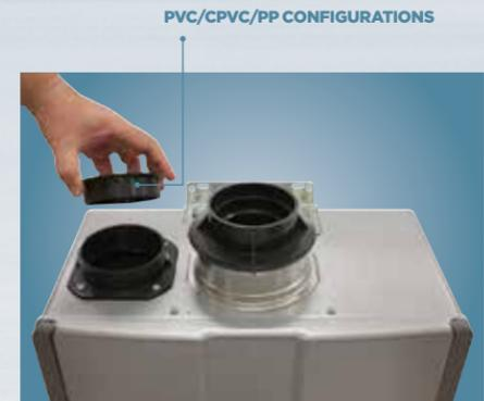
For PVC/CPVC/PP configurations, the intake cap is removed and discarded. With this option, installers can use 3- or 4-inch PVC/CPVC/PP pipe for the intake and exhaust.
