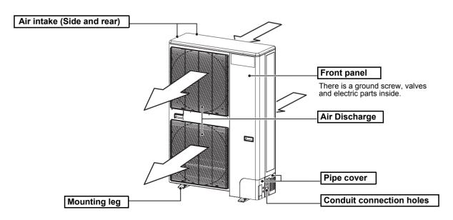
\* The image of the outdoor unit in the figure is in the case Model RAV-SP420AT2-UL.
