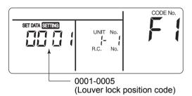
A louver number is displayed as F1, F2 on the remote control (SET DATA), showing that louver 01, 02 shown in the figure on the previous page is selected.
