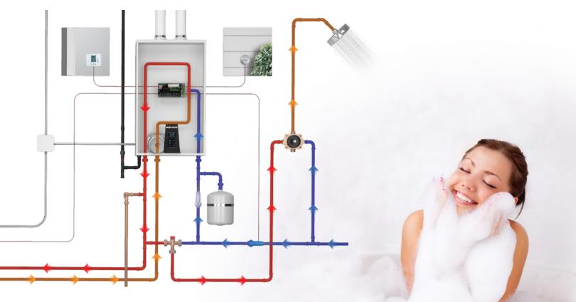
H<sub>2</sub>Air is compatible with hydronic air handler models that require W1/W2/R terminals along with single or dual-stage thermostats.\*\*
