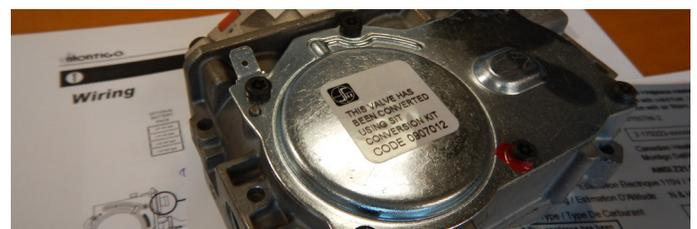
Figure 13.k Conversion label on valve
