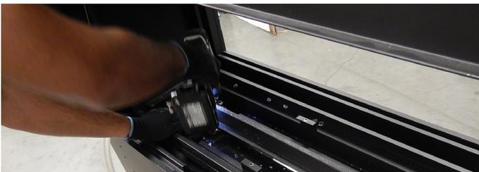
**Figure 12.d** Removing the Burner screws
