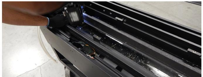
Figure 25.e. Insert burner
