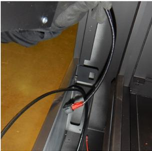
Figure 24.e On/Off switch through drawer
