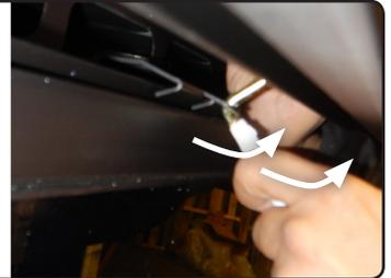
Figure 21.e Lift the latch upward
