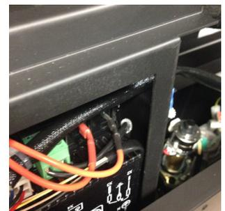
11. Valve wires are plugged into the valve in the Green, Red, and yellow ports respectively.
