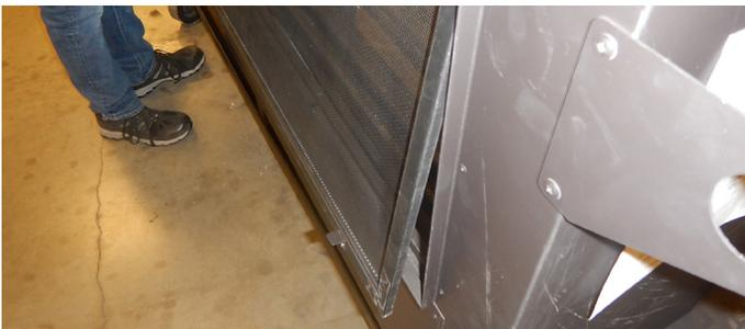
Figure 20.b Lift out the Retaining Tabs and screen
