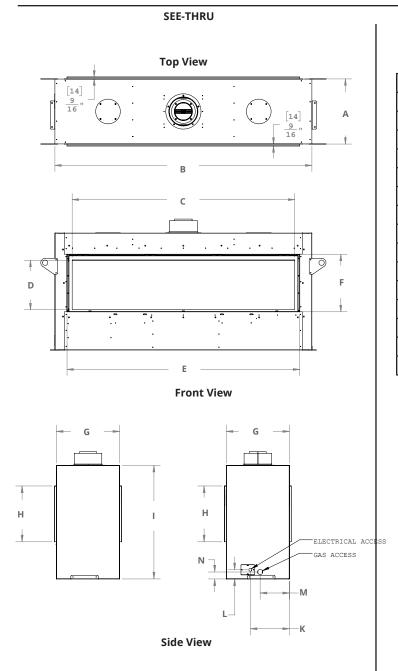
Figure 2.b DL6315ST, D6315ST Fireplace dimensions (Tolerance ± 1/8").
