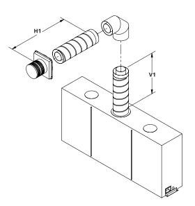
Figure 8.d Horizontal Termination - 1 Elbow
