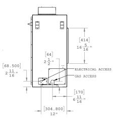
Figure 18. Gas Inlet Supply location
