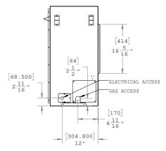
Figure 14.b Electrical Supply location on Single Sided unit
