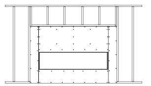
Figure 28.c non-combustible cement board with framing
