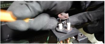
Figure 13.d Removing the spring clip
