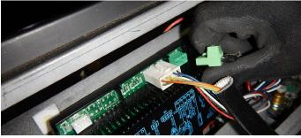
Figure 24. Remove existing basic board
