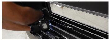
Figure 12.d Removing the Burner screws
