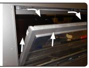
Figure 21.f Lift the door up and out of the fireplace frame
