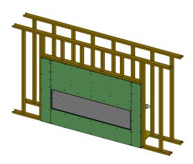
Figure 28.b non-combustible cement board with framing
