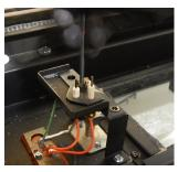
Figure 13.f Insert propane orifice, reassemble burner
