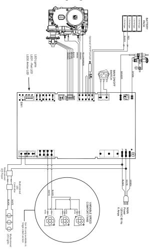
Figure 24.d D6315 (ST) (N/L) I-2 Wiring Diagram
