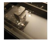
Figure 12.f Unscrewing brackets securing metal plate
