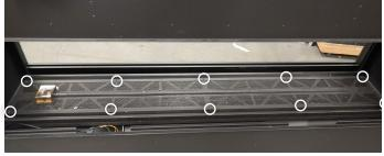
Figure 12.b Unscrewing the media trays
