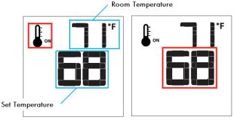
Figure 29.i Setting Room Thermostat
