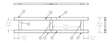
Figure 8. Assembly of Non Combustible Framing
