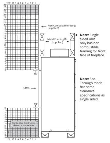
Figure 19. Combustible mantles and facings. (Not to scale)
