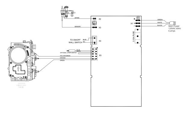
Figure 15. DL6315 (ST) (N/L) I Wiring Diagram
