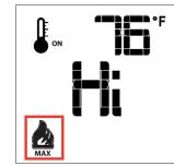
Figure 29.h Flame Level 5 and Flame Level Maximum
