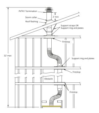
Figure 9.c Top vent, Roof mounted with 2 offsets (1 offset= two 90° bends).
