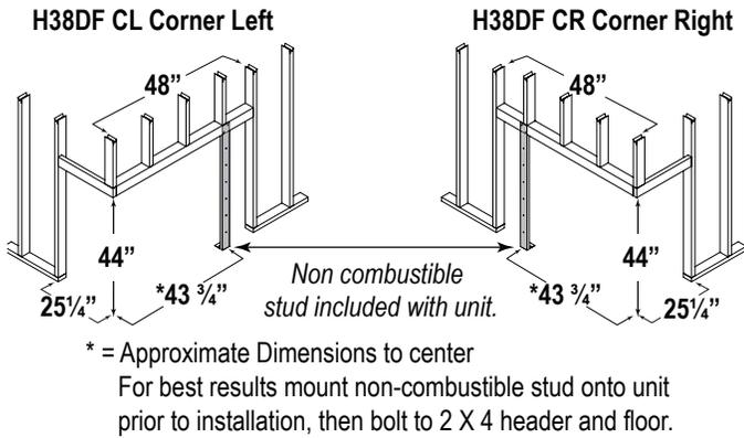
Figure 2. Framing dimensions.
