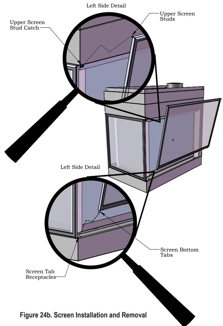
Figure 24b. Screen Installation and Removal
