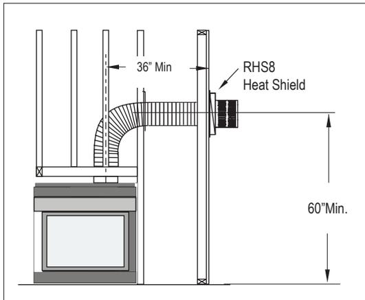
Figure 16a. RHS8 Installation. (Minimum requirements).
