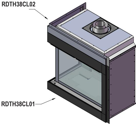
Figure 31. Replacement Door Part Codes - CL = Left
