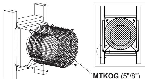
Figure 11. Installing a PTO termination heat guard.
