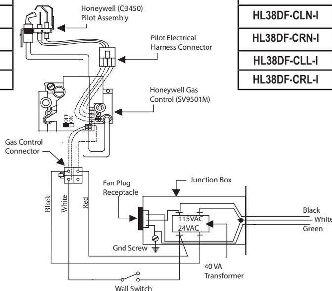
Figure 20. Wiring with Honeywell gas control and pilot.
