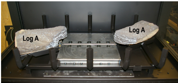
Figure 27a. Place Logs "A" on Left & Right stands.
