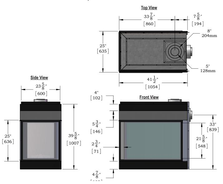
Figure 1. Fireplace dimensions with Nailing Flange Extension shown (Tolerance ± 1/8").
