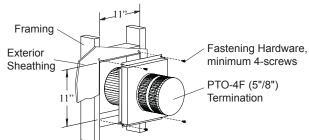
Figure 10. Installing a PTO-F termination.
