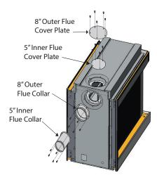
Figure 8a. Flue cover and collar installation, Rear Vented fireplace.
