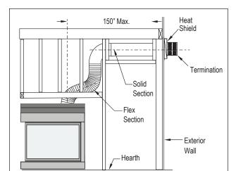
Figure 13b. H38PF\*, HL38PF\* or HP38PF\* Top Vented, wall mounted Multi-elbow installation. See Venting Graph for Top vent, wall mounted
