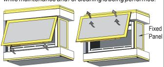
Figure 25g. Removing and installing the glass doors. (Both Sides Typical)
