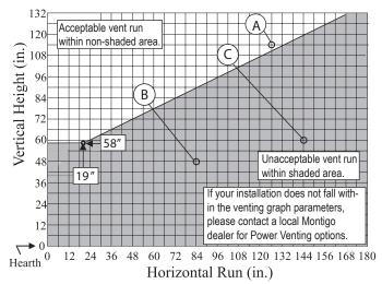
Figure 13. HP38PF\* Top Vent Venting Graph for wall mounted terminations.
