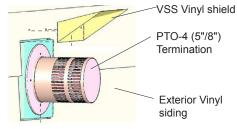
Figure 10d. Installing the VSS Vinyl Shield.
