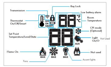
Figure 29b. Remote Control LCD Display
