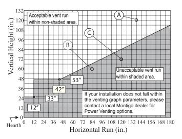
Figure 14. H38PF\* or HL38PF\* Rear Vent Venting Graph for wall mounted terminations.
