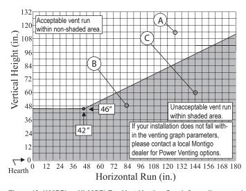
Figure 12. H38PF\* or HL38PF\* Top Vent Venting Graph for wall mounted terminations.
