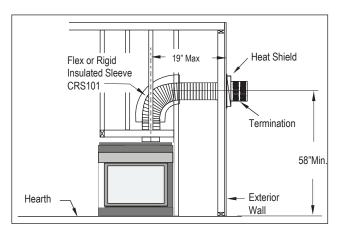
Figure 13a. HP38PF\* Top Vented, wall mounted installation with one 90° bend. The vent run must comply with Venting Graph for Top vent, wall mounted terminations, Figure 13.
