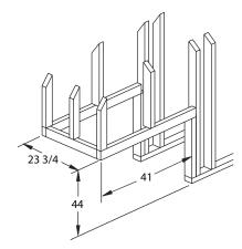
Figure 2. Framing dimensions.
