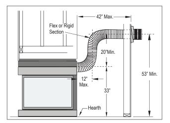
Figure 15a. H38PF\* or HL38PF\* Rear Vented, wall mounted Multi-elbow termination installation. The vent run must comply with the Venting Graph for Rear vent, wall mounted terminations, Figure 14.
