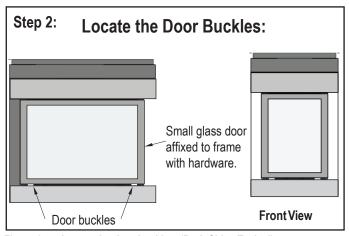
Figure 25a. Locate the door buckles. (Both Sides Typical)
