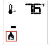
Figure 29f. Flame Off and Flame Level 1.
