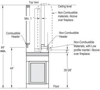
Figure 5. Non Combustible Framing with alcove above fireplace, Top Vent.
