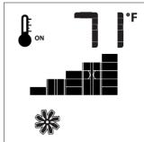
Figure 29I. Fan Speed Control
