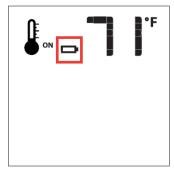
Figure 29p. Low Battery Power Detection
