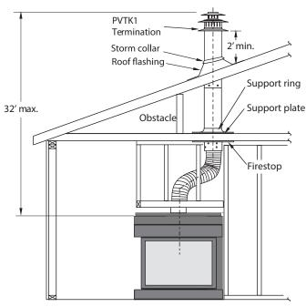
Figure 9a. Top vent, Roof mounted with 1 offset (1 offset= two 90°
