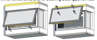
Figure 25g. Removing and installing the glass door.
