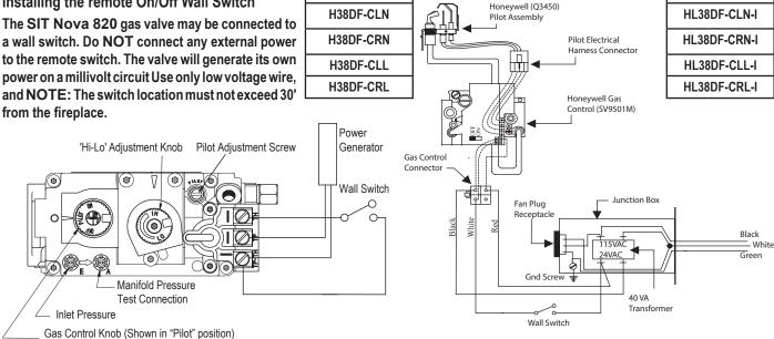
Figure 19. Wiring with SIT Nova 820.
