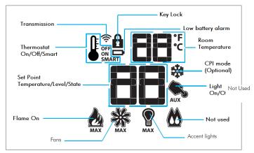
Figure 29b. Remote Control LCD Display
