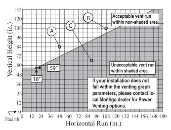
Figure 14a. HP38C\* Rear Vent Venting Graph for wall mounted terminations.
