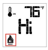
Figure 29g. Flame Level 5 and Flame Level Maximum.
