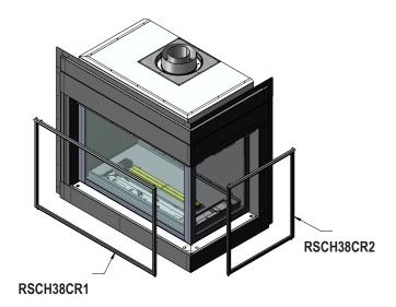
Figure 31c. Replacement Screen Part Codes - CR = Right
