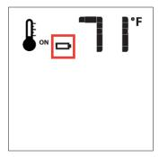
Figure 29p. Low Battery Power Detection
