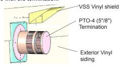
Figure 10d. Installing the VSS Vinyl Shield.
