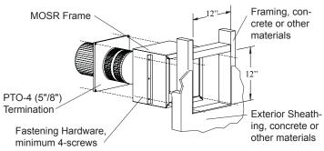
Figure 10c. Installing a PTO termination with the MOSR frame.
