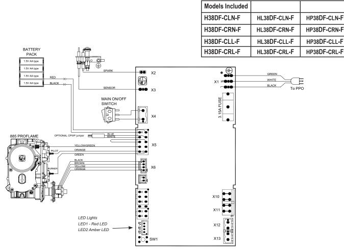
Figure 18. Wiring Diagram for the SIT Proflame 2 Electronic Ignition with remote control
