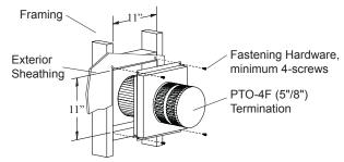
Figure 10. Installing a PTO-F termination.
