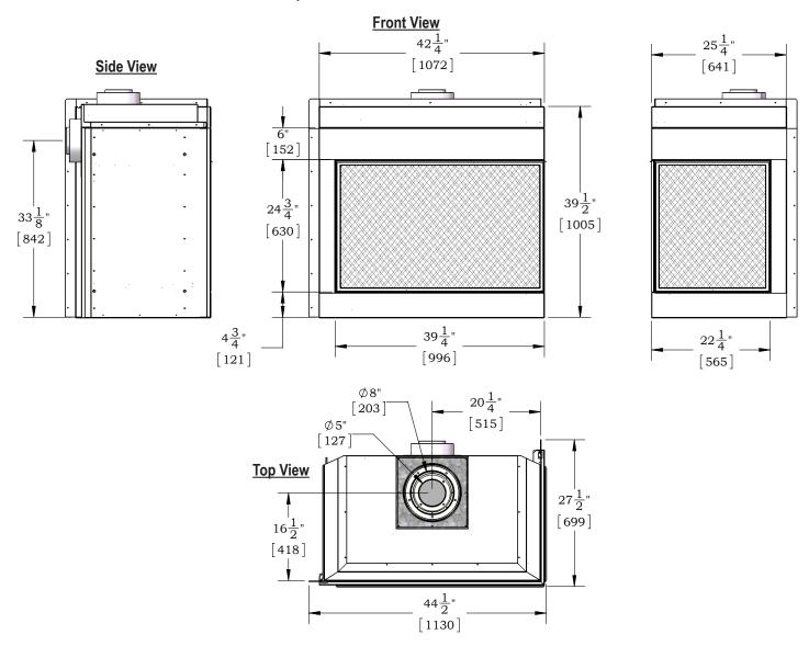
Figure 1. Fireplace dimensions with attached Nailing Flange for Corner Left shown, Fireplace dimensions same for corner right. (Tolerance  $\pm \frac{1}{8}$ ").
