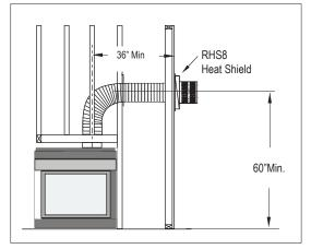
Figure 16a. RHS8 Installation. (Minimum requirements).
