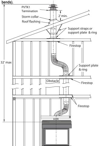
Figure 9b. Top vent, Roof mounted with 2 offsets (1 offset= two 90° bends).
