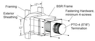
Figure 10b. Installing a PTO termination with the BSR frame.
