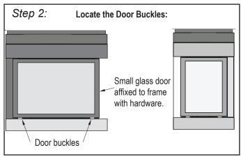
Figure 25a. Locate the door buckles.
