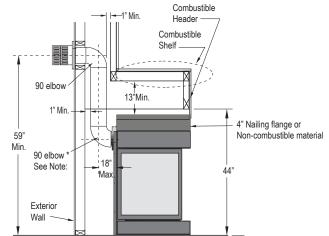
Figure 4. Combustible Framing for shelves over the fireplace, Rear vent.
