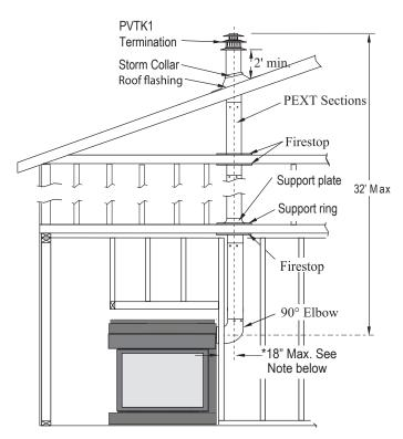
Figure 9c. Rear vent, Roof mounted venting (1 = 90° bend).
