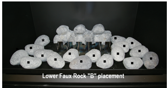
Figure 33e. Placement of (17) seventeen Lower "B" faux ceramic rocks. Note approximate location and placement. (Do not cover the burner holes if possible). (Place one of the rocks on top of the Pilot cover *).
