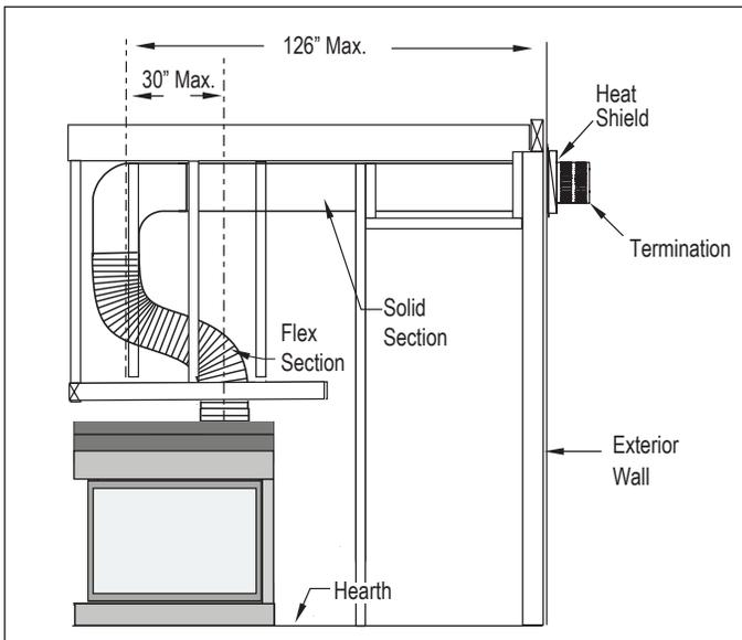
Figure 13b. H38PF\* , HL38PF\* or HP38PF\* Top Vented, wall mounted Retracted Multi-elbow installation. See Venting Graph for Top vent, wall mounted terminations, Figure 12 or 13.
