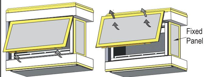
Figure 25g. Removing and installing the glass doors. (Both Sides Typical)
