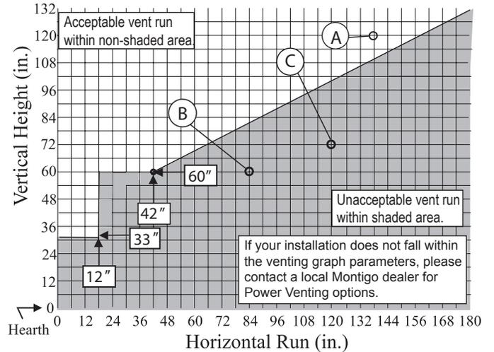
Figure 14a. HP38PF\* Rear Vent Venting Graph for wall mounted terminations.
