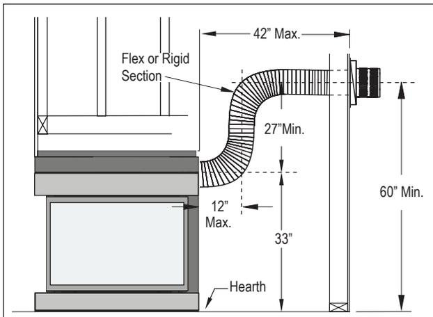
Figure 15b. HP38PF\* Rear Vented, wall mounted Multi-elbow termination installation. The vent run must comply with the Venting Graph for Rear vent, wall mounted terminations, Figure 14a.
