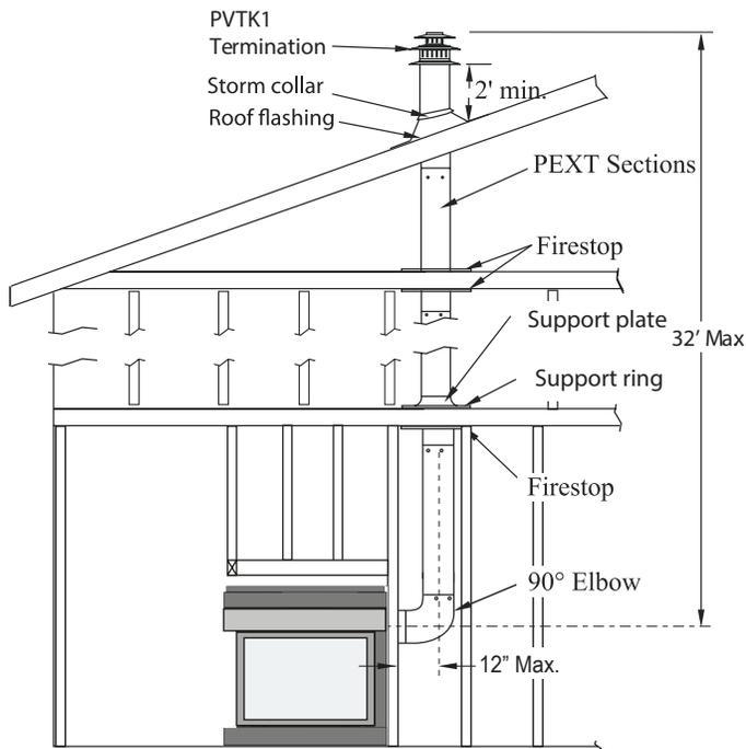
Figure 9c. Rear vent, Roof mounted venting (1 = 90° bend).
