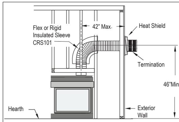
Figure 12a. H38PF\* or HL38PF\* Top Vented, wall mounted installation with one 90° bend. The vent run must comply with Venting Graph for Top vent, wall mounted terminations, Figure 12.
