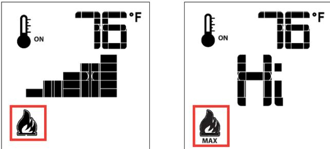
Figure 29g. Flame Level 5 and Flame Level Maximum.
