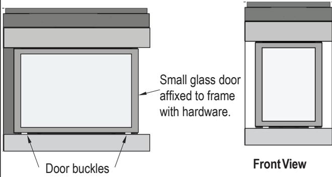
Figure 25a. Locate the door buckles. (Both Sides Typical)
