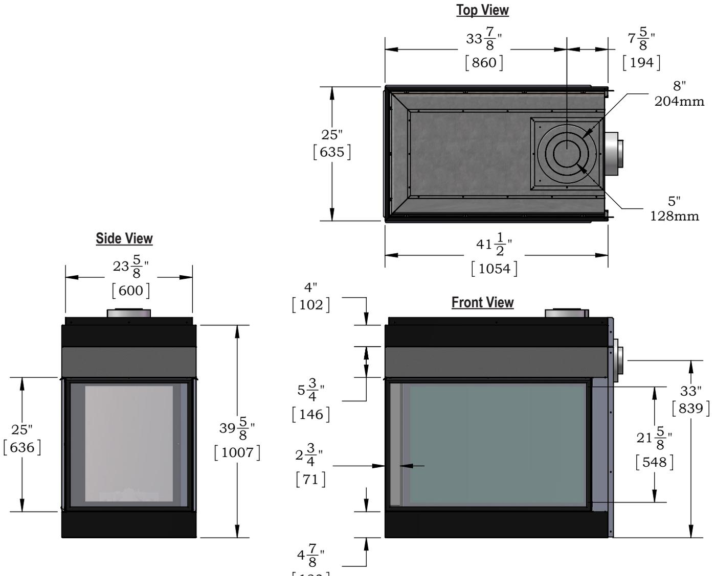
Figure 1. Fireplace dimensions with Nailing Flange Extension shown (Tolerance  $\pm \frac{1}{8}$ ").
