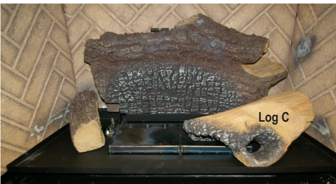
Figure 31c. Placing front logs.
