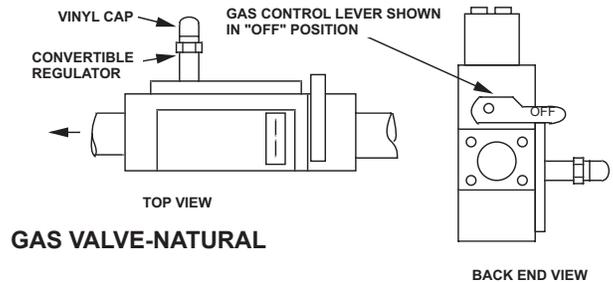
**Warning: Conversion must be done by a qualified service technician. Main burner orifice(s) and new gas conversion label are provided in conversion kit attached to manifold pipe.**
