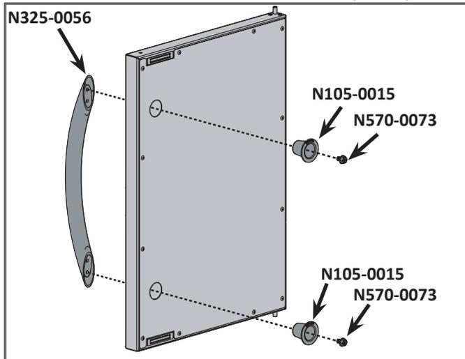
The door handle is not mounted for shipping purposes. It must be mounted to the outside surface of the door as illustrated.
