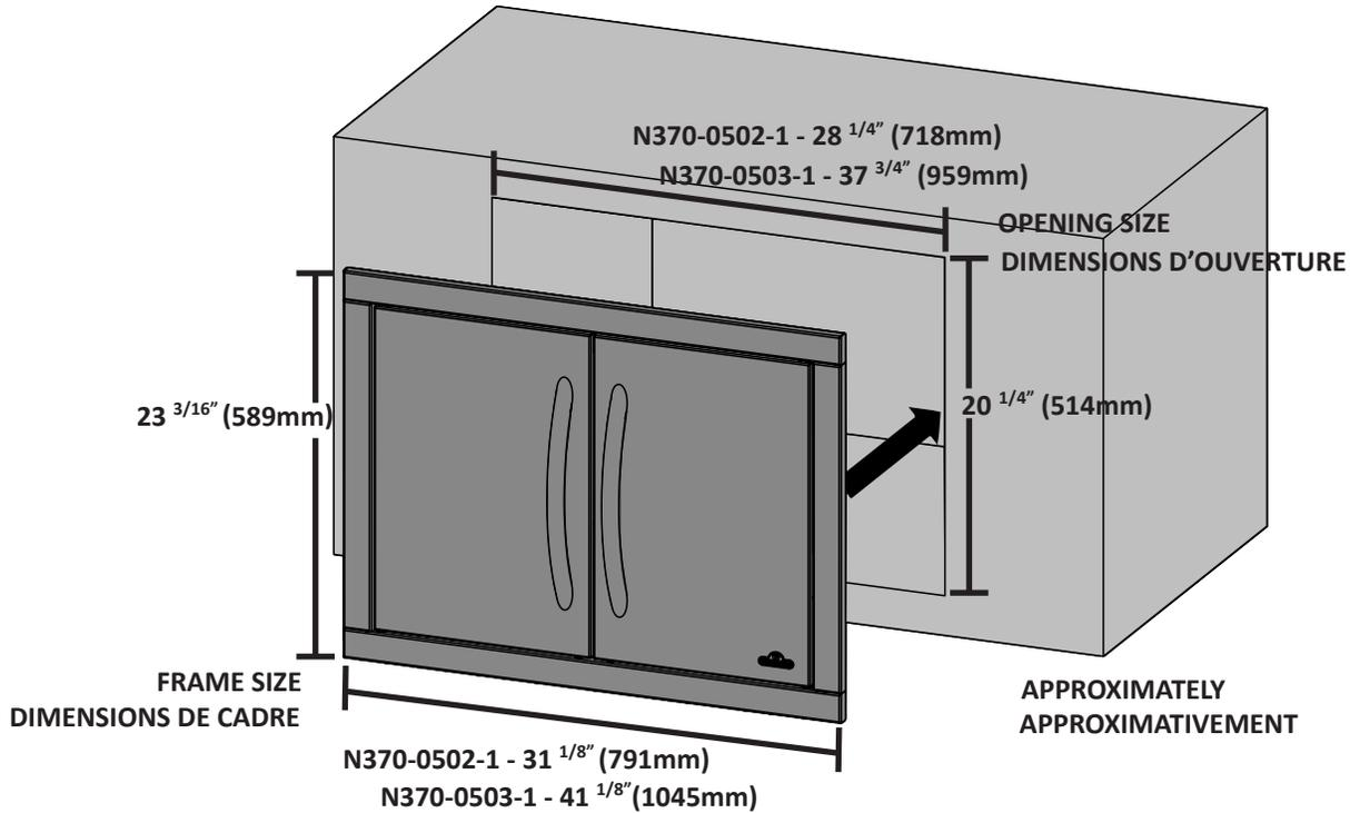
The door opening required for the stainless steel double door accessory kit is as shown. The frame must be mounted in the cabinet level horizontally and vertically for the doors to close properly. The door frame must be installed squarely to prevent uneven gaps between the doors and frame. Check for squareness by measuring diagonally across the frame in both directions. Once these two measurements are equal to each other, the frame is to be considered square.
