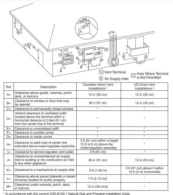
In accordance with the current CSA B149.1 Natural Gas and Propane Installation Co
