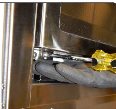
Figure 60 Removing the left side screw
