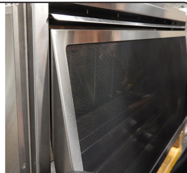
Figure 62 Lifting the base of the door
