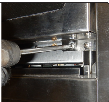
Figure 61 Removing the right side screw
