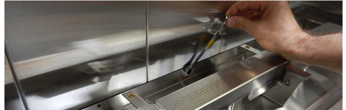
Figure 52 Loosening air baffle bolts
