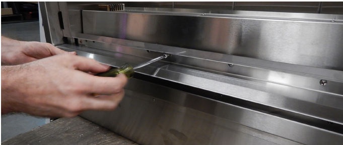
Figure 4 Removal of lower air baffle
