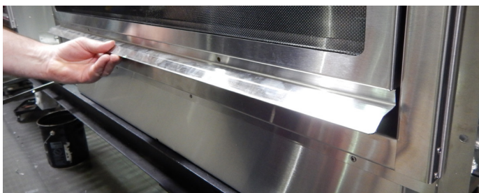
Figure 59 Removing the left side screw
