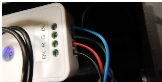
Figure 48 Wiring the LED receiver
