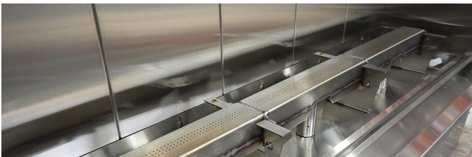
Figure 51 Firebox with tray removed
