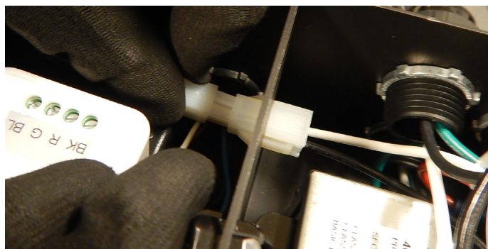
Figure 47 Connecting the LED receiver
