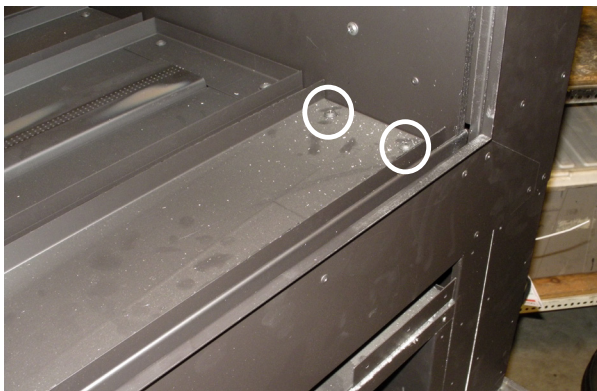
Figure 11a. Removing screws that secure media tray
