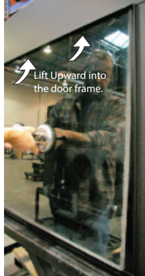
Figure 7b. (Lift the door upward)
