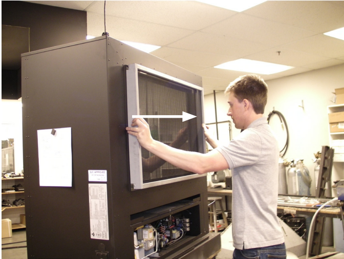
Figure 7. Removing the screen
