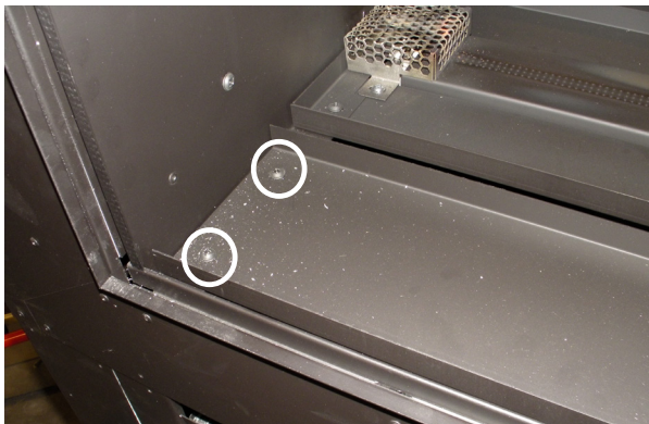
Figure 11. Removing screws that secure media tray
