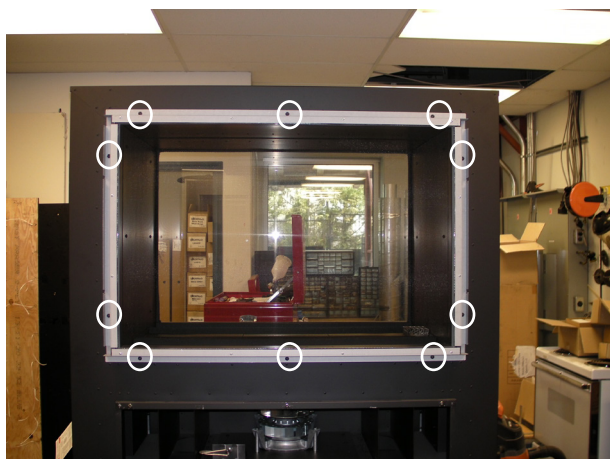
Figure 7g. Removing screws that secure screen.
