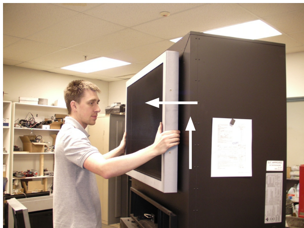
Figure 7e. Lifting screen frame up and out.
