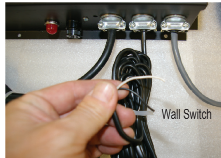
Figure 15c. (Wall Switch Wire connection)
