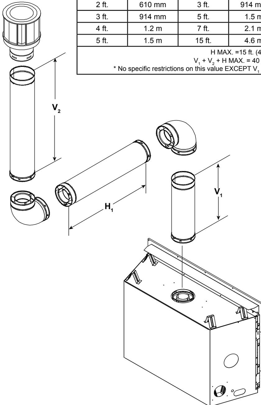
**Note:** There **MUST** be a 25% reduction in total H when using SLP-FLEX Series (6-5/8 inch) vent except when using the simple up and out installation. See Figure 4.8.
