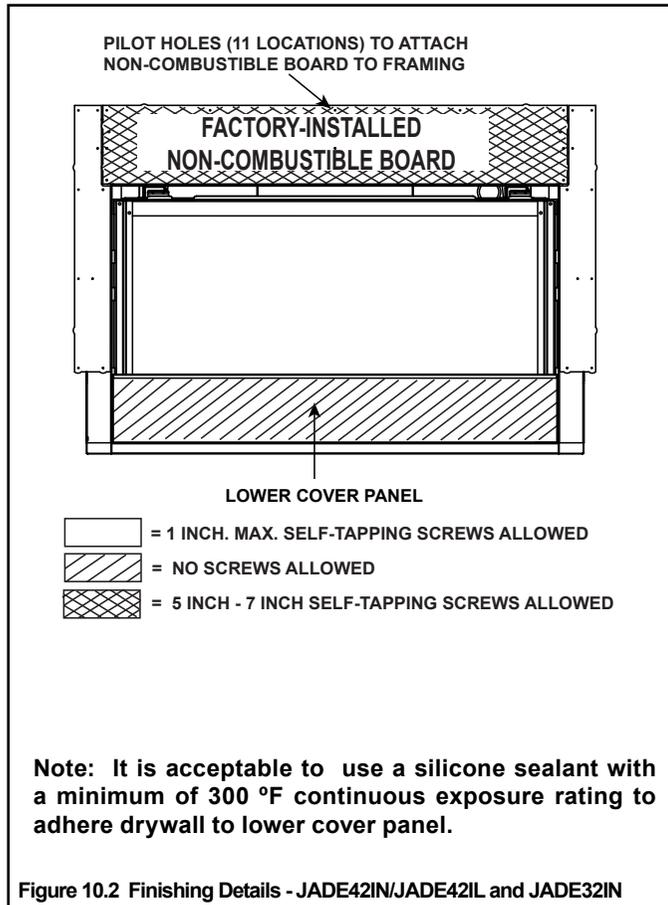
**CAUTION! Risk of Glass Damage and Cuts!** DO NOT drill or install any type of screw or fastener into the lower cover panel. Sharp screw or fastener tips may penetrate and break the glass or cause cuts.
