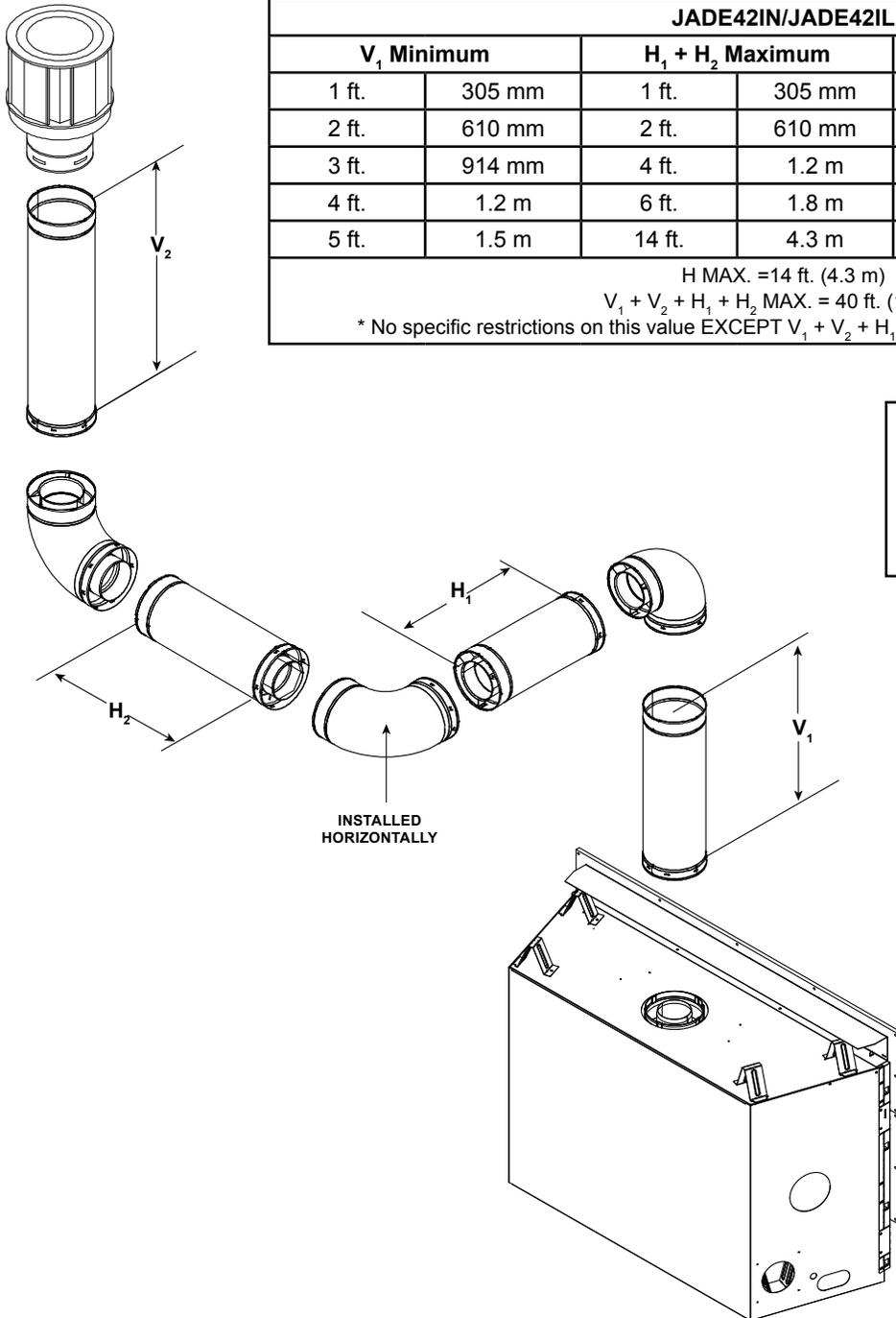
**Note:** There MUST be a 25% reduction in total H when using SLP-FLEX Series (6-5/8 inch) vent except when using the simple up and out installation. See Figure 4.8.
