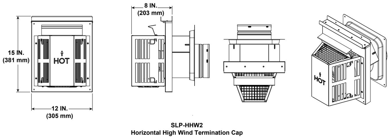
Figure 12.4 SLP series Vent Components
