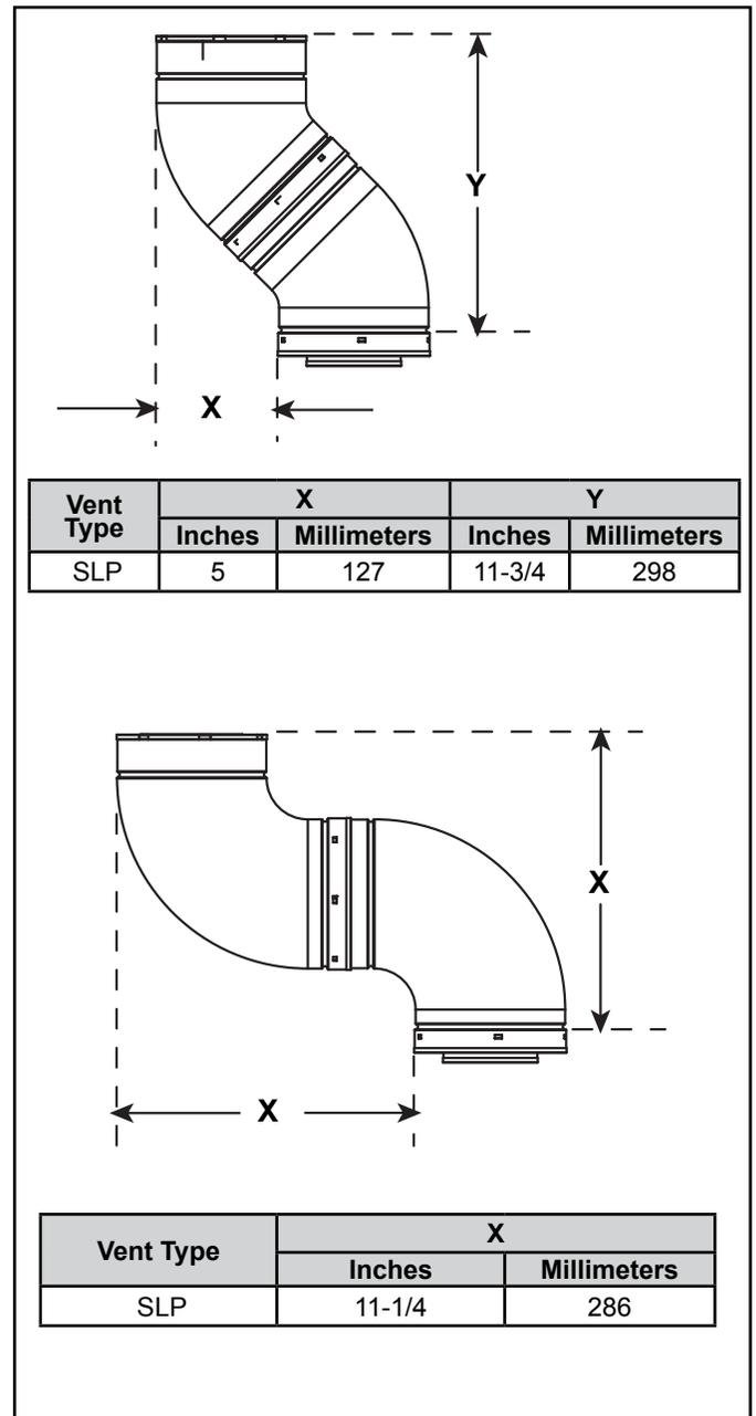
Figure 4.5 Vertical and Horizontal Offset for SLP Elbows
