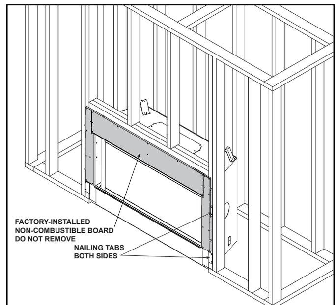
**Figure 6.5 Proper Positioning, Leveling And Securing Of Appliance**
