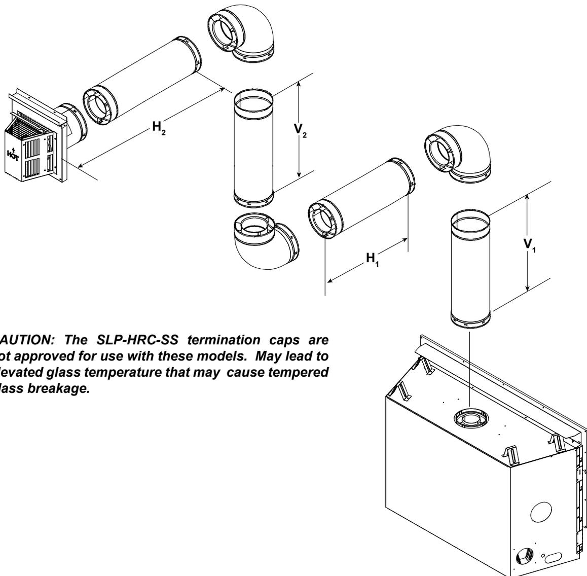
**CAUTION:** The SLP-HRC-SS termination caps are not approved for use with these models. May lead to elevated glass temperature that may cause tempered glass breakage.
