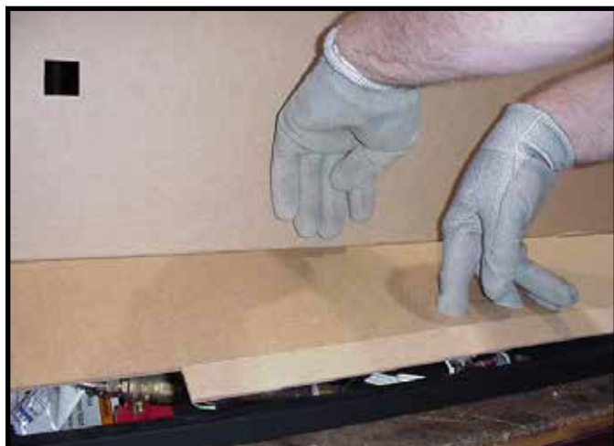
Figure 11.9 Opening Lower Access Panel
