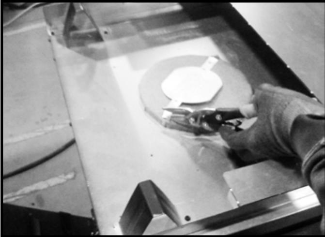
Figure 6.1 Cut the metal retaining band and fold the sides out.
