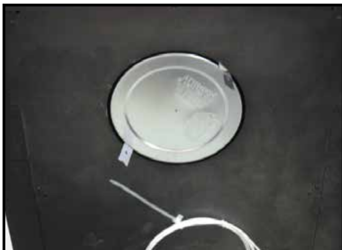
Figure 6.5 Remove the seal cap.
