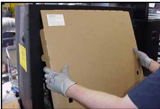
Figure 11.5 Installation of Splatter Guard
