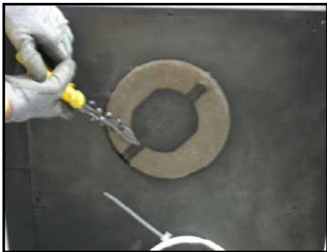
Figure 6.4 Cut the metal retaining band.
