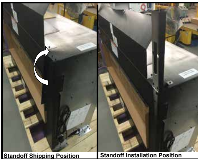
Figure 6.1 Standoffs Shown in Vertical Position
