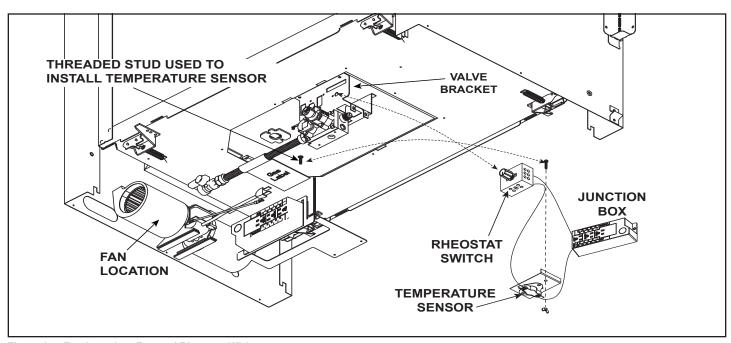
Figure 8.4 Fan Location, Fan and Rheostat Wiring
