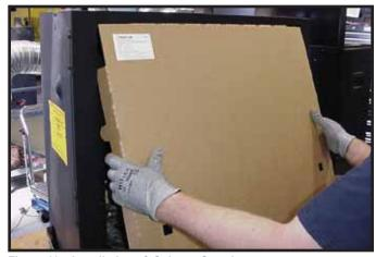
Figure 11.5 Installation of Splatter Guard
