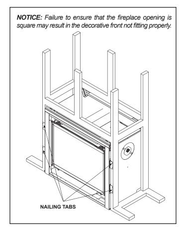
Figure 6.11 Securing An Appliance
