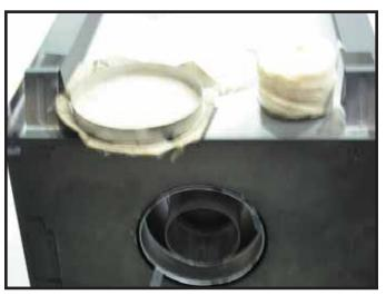
**Figure 6.8** Discard the seal cap, insulation plug and the insulation basket.
