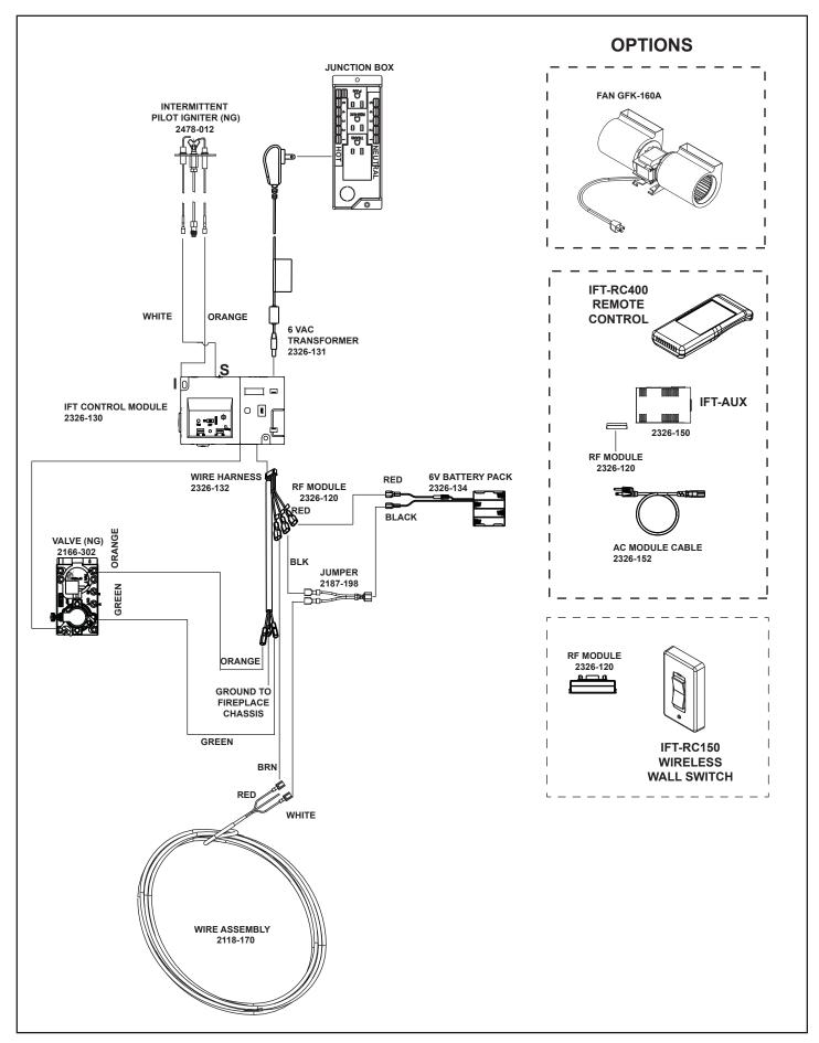
Figure 8.2 IntelliFire™ Touch Wiring With Wall Switch
