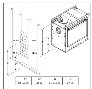
Shows center of vent framing hole for top or rear venting. The center of the hole is one (1) inch (25.4 mm) above the center of the horizontal vent pipe.
