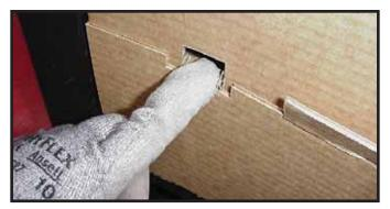
Figure 11.10 Securing Tabs Inside Front of Splatter Guard
