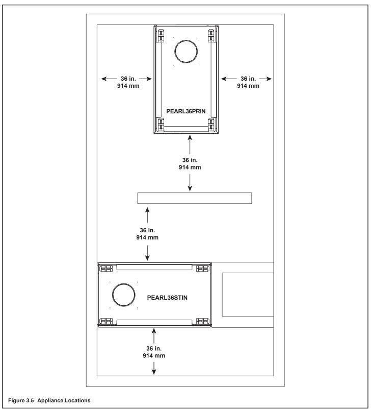
**NOTICE:** Install appliance on hard metal or wood surfaces extending full width and depth. **DO NOT** install directly on carpeting, vinyl, tile or any combustible material other than wood.
