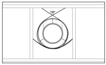
Figure 7.9 Securing Horizontal Pipe Sections
