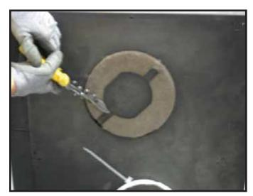
Figure 6.6 Cut the metal retaining band.
