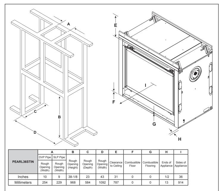
Adjust framing dimensions for interior sheathing (such as sheetrock)
