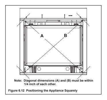
Figure 6.10 Proper Positioning and Leveling of an Appliance
