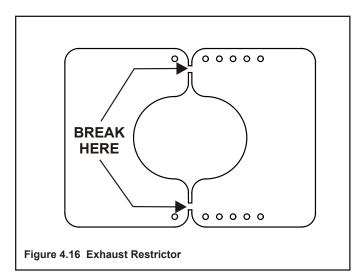
3. Use Table 4.1 to match the amount of vertical you have in the system to find the appropriate position to set the exhaust restrictor. See Figure 4.17.
