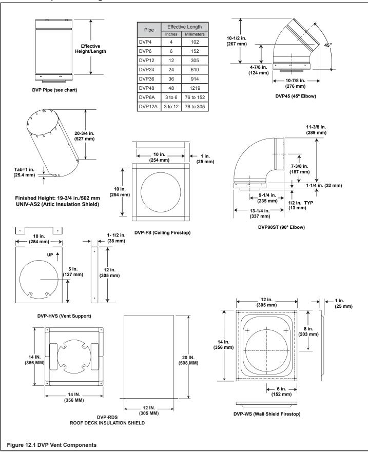
Note: Heat shields MUST overlap by a minimum of 1-1/2 in. (38 mm). The heat shield is designed to be used on a wall 4 in. to 7-1/4 in. (102 mm to 184 mm) thick. If wall thickness is less than 4 in. (102 mm) the existing heat shields must be field trimmed. If wall thickness is greater than 7-1/4 in. (184 mm) a DVP-HSM-B will be required.
