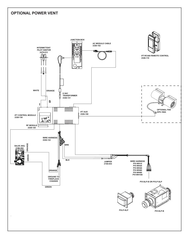
Figure 8.3 IntelliFire™ Touch Wiring With Optional Power Vent
