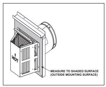
Figure 4.6 Measure to Outside Mounting Surface
