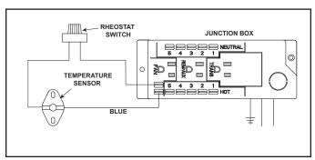
Figure 8.5 Detail of Fan Wiring with Rheostat
