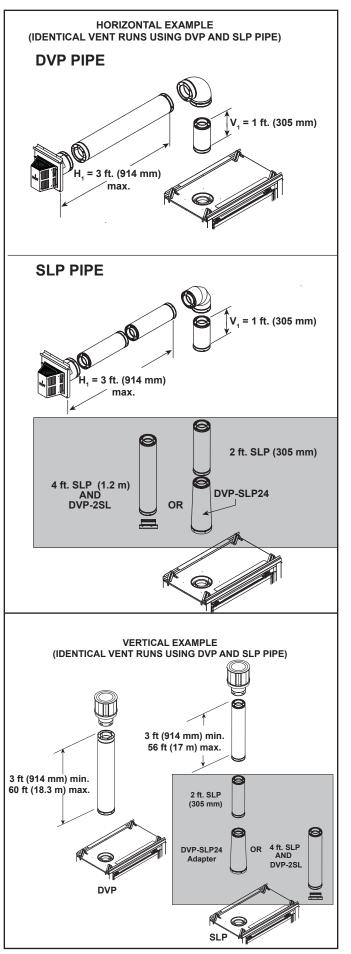
Figure 4.9 Adapt DVP Pipe to SLP Using DVP-SLP24 & DVP-2SL
