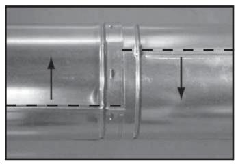
Figure 7.10 Rotate Seams for Disassembly
