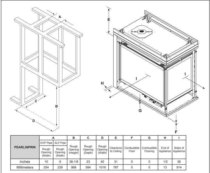
Adjust framing dimensions for interior sheathing (such as sheetrock)
