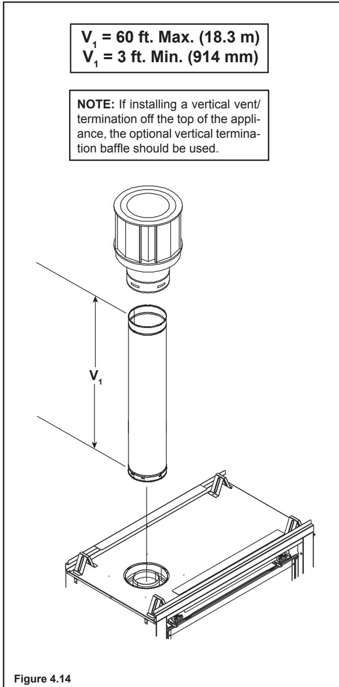
Exhaust restrictors are recommended for these vertically terminated products which have excessive draft. Exhaust restrictors will compensate for high draft, and restore visual flame height. If the vent configuration has a total vertical of 10-60 feet, an exhaust restrictor may be needed. The exhaust restrictor can be located in the appliance manual bag.
