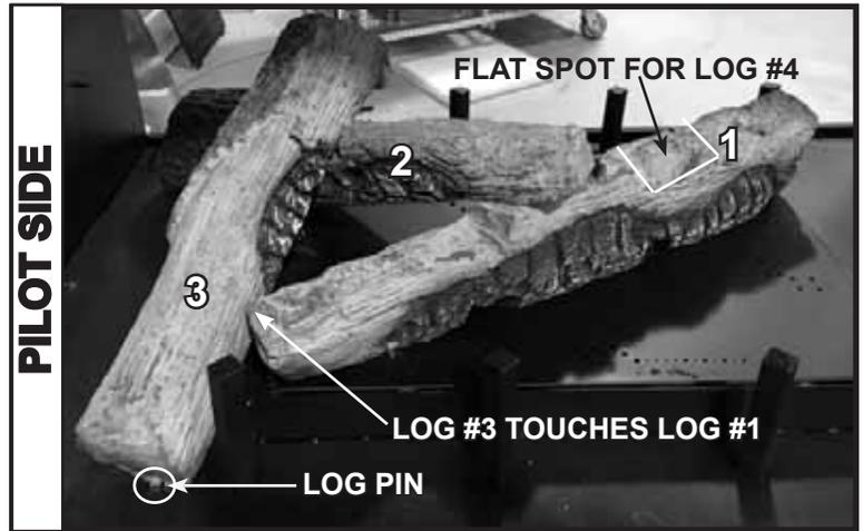
Figure 5. Log #3 Installed
