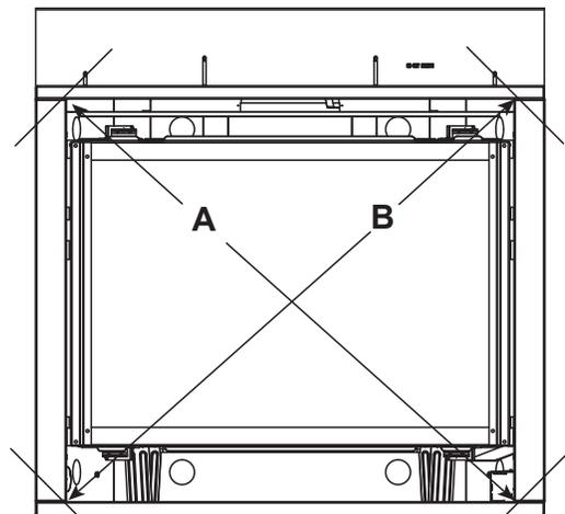
Note: Diagonal dimensions (A) and (B) must be within 1/4 inch of each other.
