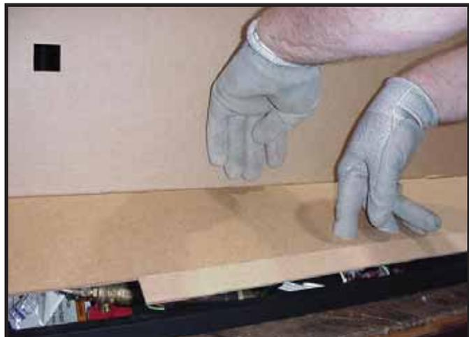
Figure 11.9 Opening Lower Access Panel
