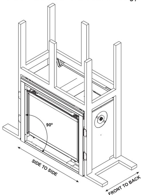
Figure 6.10 Proper Positioning and Leveling of an Appliance
