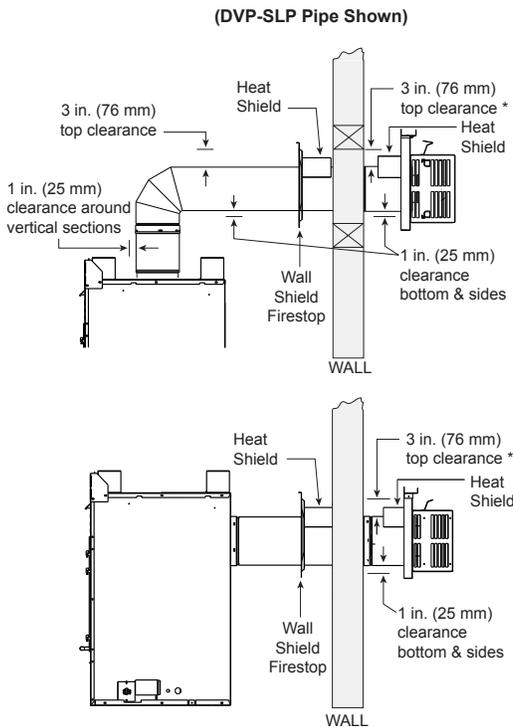
\* When using SLP pipe, minimum clearances from the vent pipe to combustible materials at inside wall firestops are:
