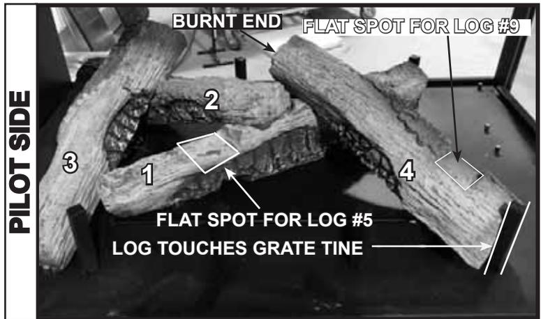
Figure 6. Log #4 Installed
