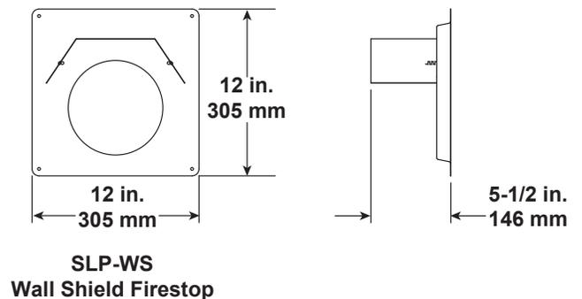
Figure 12.8 SLP Series Vent Components
