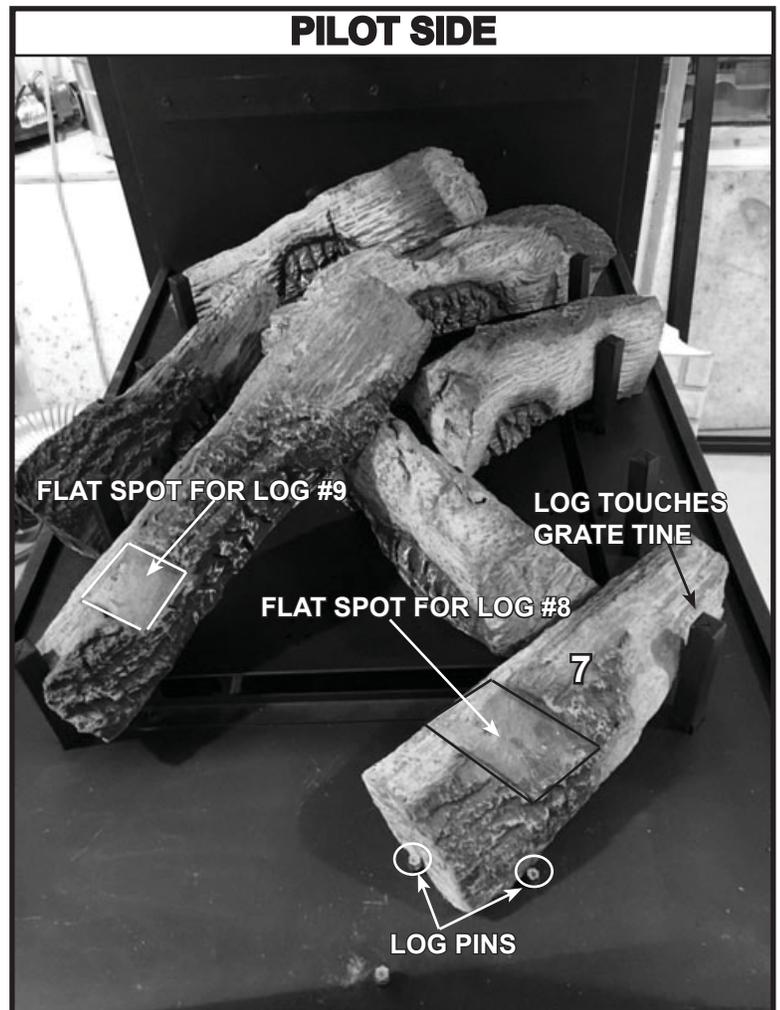
Figure 9. Log #7 Installed
