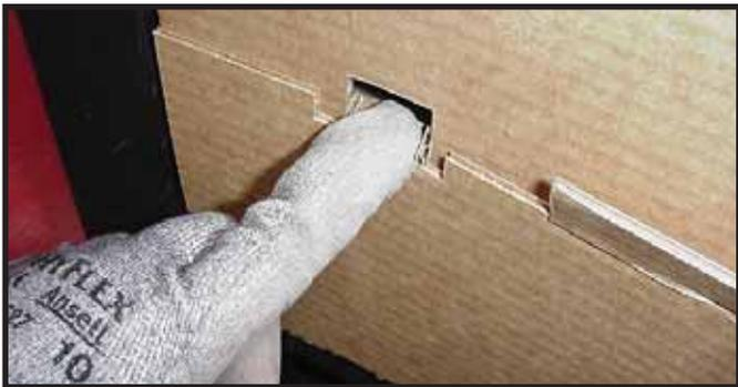
Figure 11.10 Securing Tabs Inside Front of Splatter Guard
