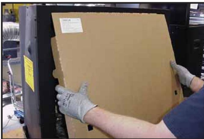
Figure 11.5 Installation of Splatter Guard
