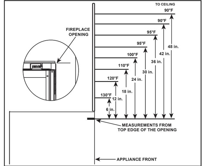
Figure 2.1 Good Faith Wall Surface Temperatures Above Appliance
