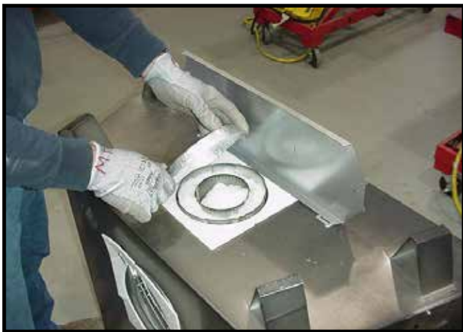
Figure 6.8 Remove the seal cap.
