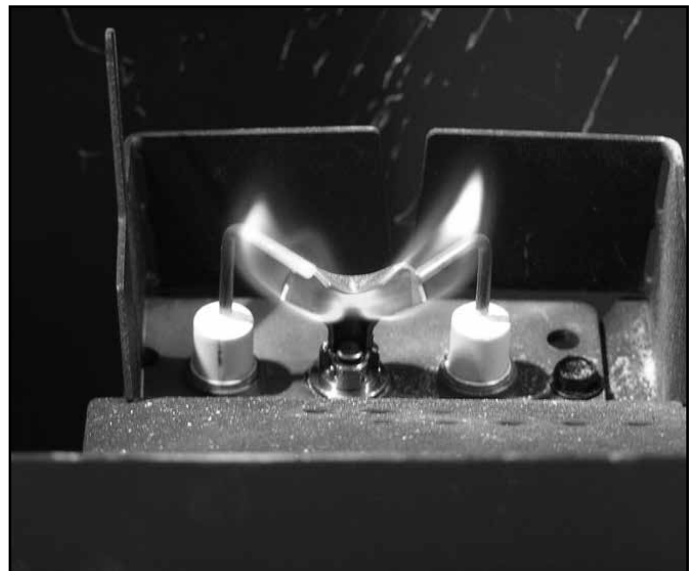
Figure 3.1 IPI Pilot Flame Patterns
