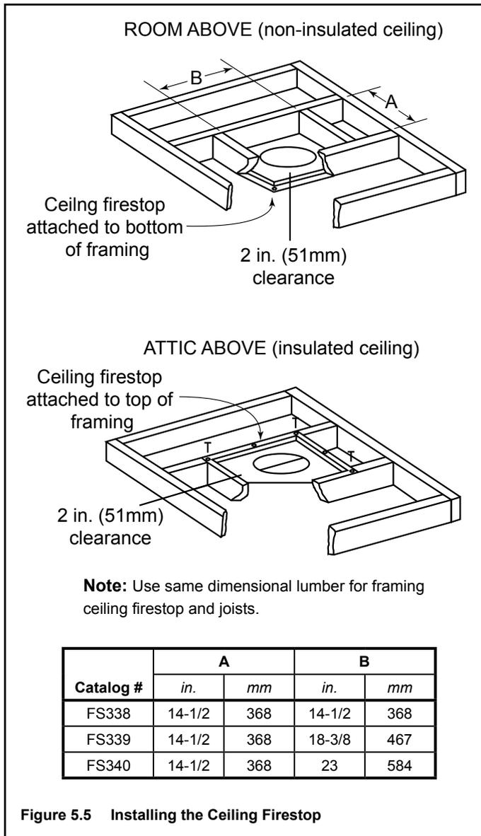
**WARNING! Risk of Fire! DO NOT** seal area between firestop opening and chimney pipe except where they enter the attic or leave the warm air envelope of the home (use 600° F sealant).
