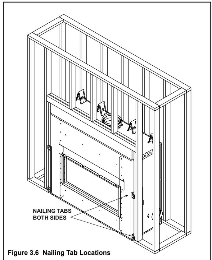
Figure 3.6 Nailing Tab Locations
