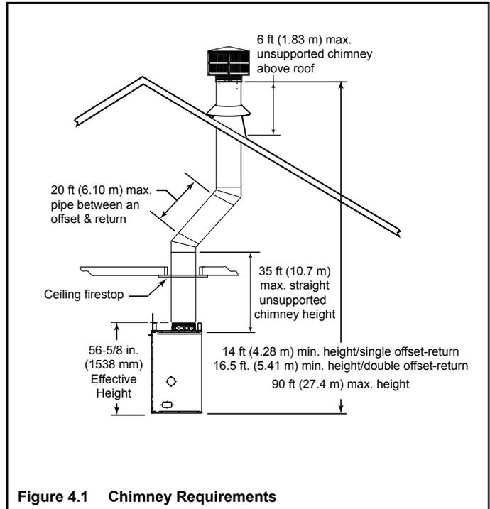
**Figure 4.1 Chimney Requirements**
