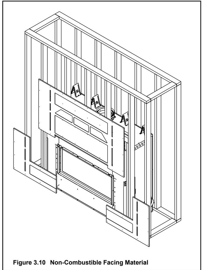
Figure 3.10 Non-Combustible Facing Material
