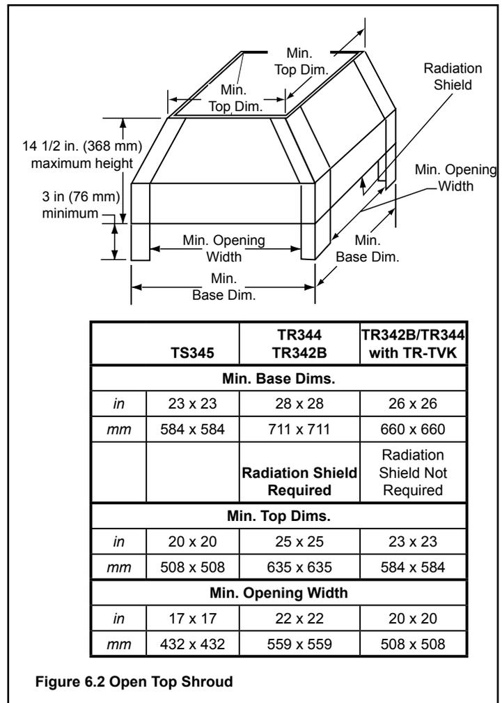
TR caps require radiation shield unless installed partially above the shroud or using a TR-TVK. The TR cap must be raised to the minimum dimensions (or greater) above the shroud. Refer to Figure 6.3.
