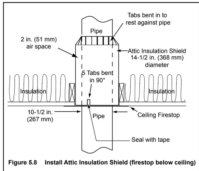
Figure 5.8 Install Attic Insulation Shield (firestop below ceiling)
