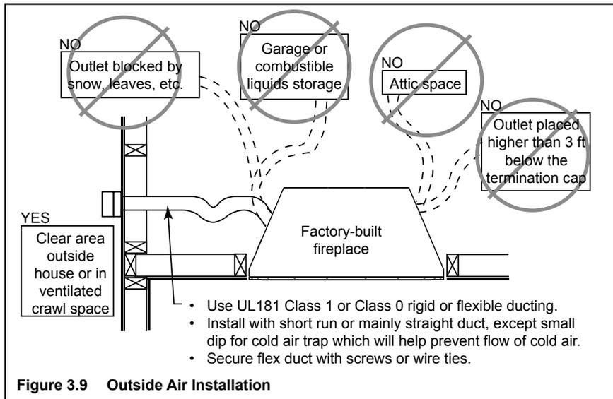
Figure 3.9 Outside Air Installation
