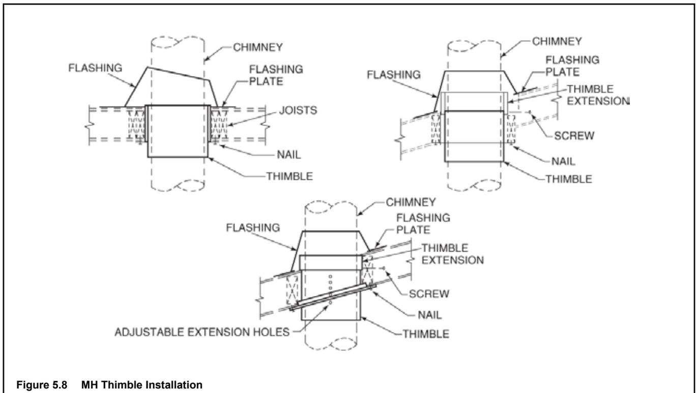
Figure 5.8 MH Thimble Installation
