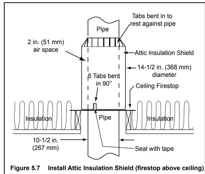
Figure 5.7 Install Attic Insulation Shield (firestop above ceiling)
