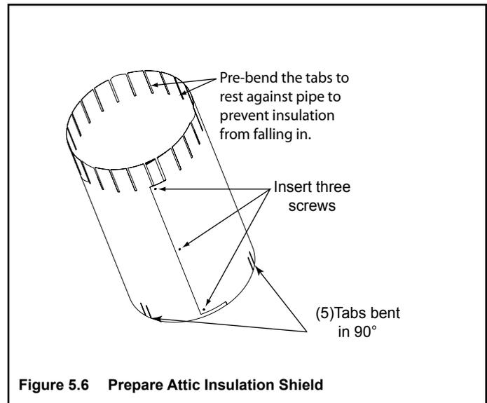
Figure 5.6 Prepare Attic Insulation Shield
