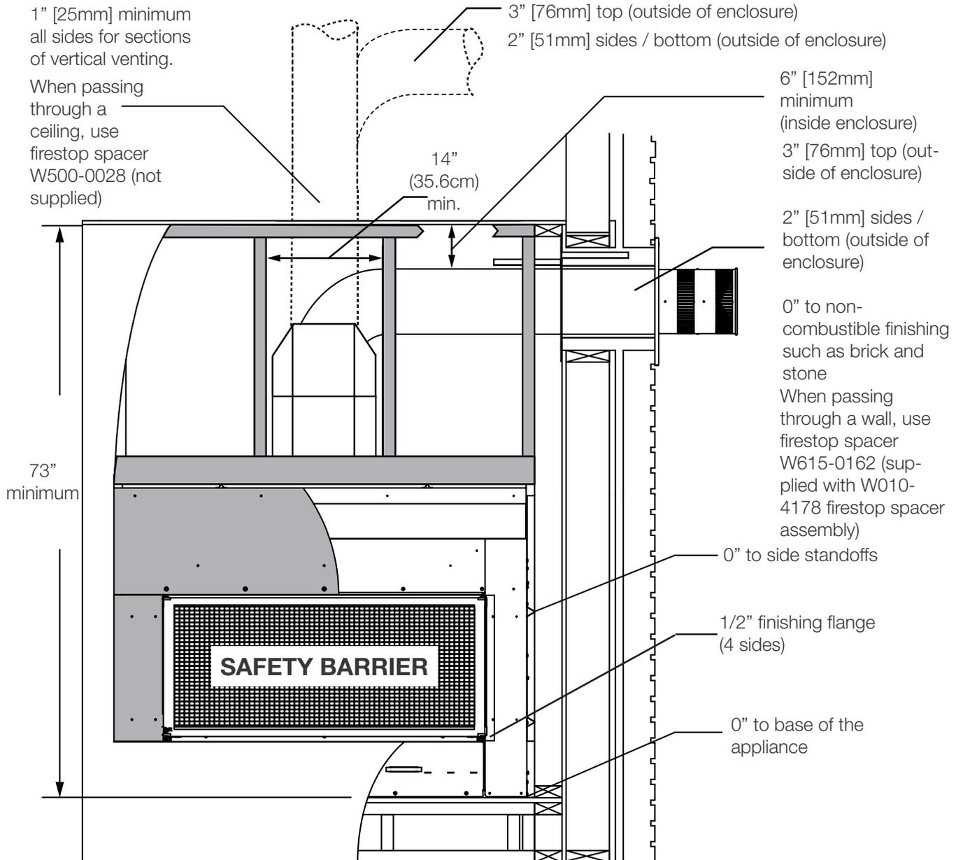
**Horizontal vent sections:** A minimum clearance of 3" (76mm) on the top outside of the enclosure and 2" (51mm) on the sides and bottom outside of the enclosure all around the vent pipe on all horizontal runs to combustibles is required. Horizontal vent sections within enclosures require a minimum clearance of 6" (152mm) at the top of the vent pipe.
