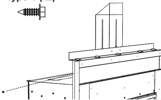
Secure with screw supplied in the manual baggie to the upper front frame
