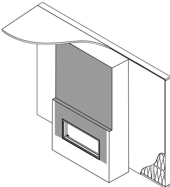
**SHADED AREA MUST BE NON-COMBUSTIBLE MATERIALS.** Recessed installation **requires** recess material to use non-combustible facing due to close proximity to vent.
