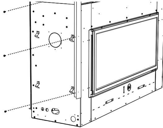
Align the nailing tab with the holes on the appliance then secure with the screws removed in step 1.
