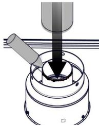
USE RED SILICONE TO SEAL REDUCER TO THE AIR INTAKE COLLARS.
