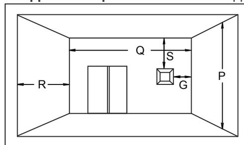
$$Q_{\text{MIN}} = 3 \text{ feet (0.9m)} \quad R_{\text{MAX}} = 2 \times Q_{\text{ACTUAL}} \quad R_{\text{MAX}} \leq 15 \text{ feet (4.6m)}$$
