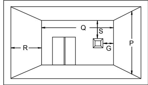
$$Q_{\text{MIN}} = 3 \text{ feet (0.9m)} \quad R_{\text{MAX}} = 2 \times Q_{\text{ACTUAL}} \quad R_{\text{MAX}} \leq 15 \text{ feet (4.6m)}$$
