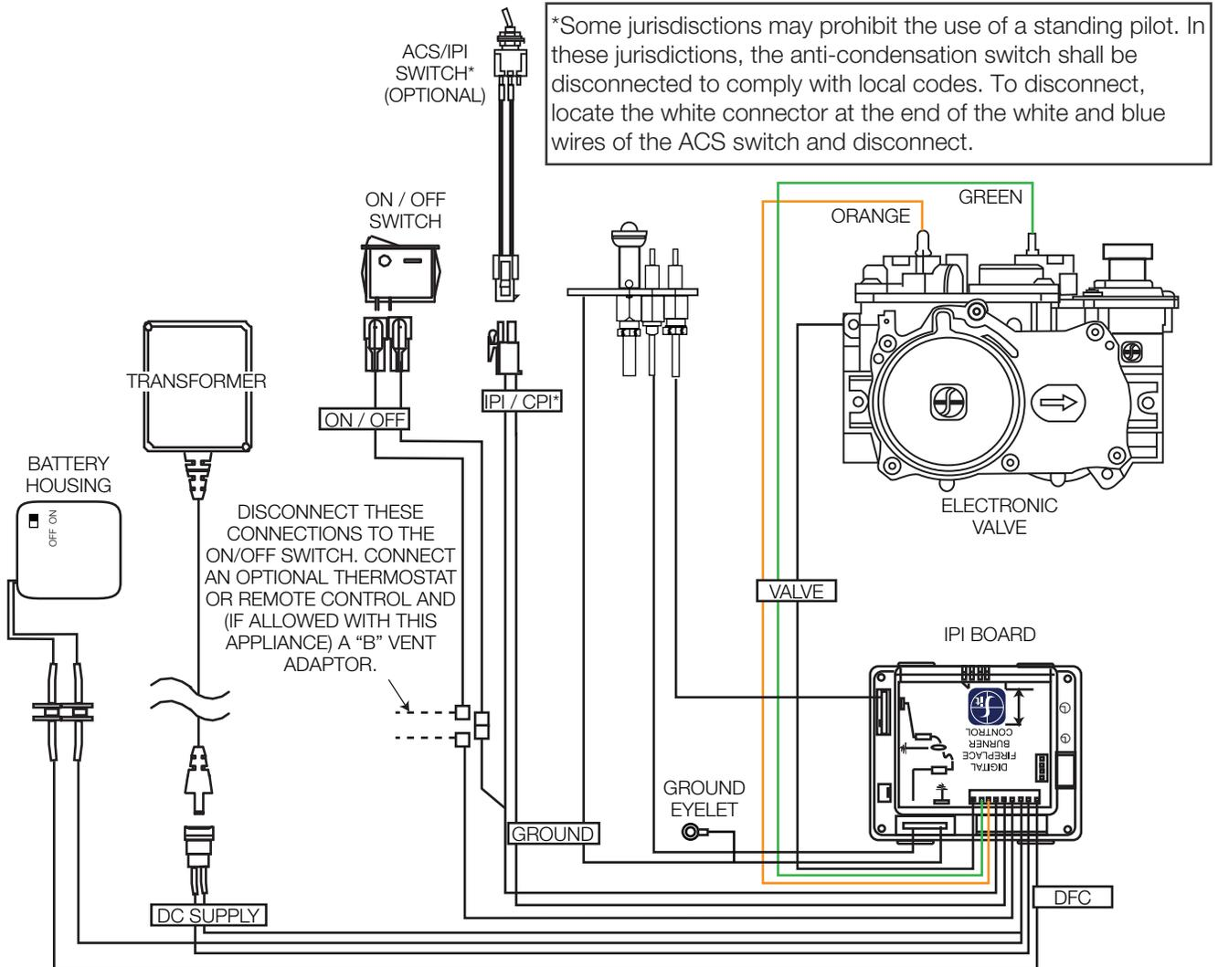
WHERE APPLICABLE, APPLIANCES WITH "B" VENT ADAPTORS MUST HAVE THE SPILL SWITCH WIRED IN SERIES WITH EITHER THE EXISTING SWITCH OR OPTIONAL WALL SWITCH, THERMOSTAT OR REMOTE.
