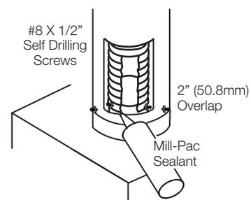
**4.3.4 horizontal air terminal installation**
