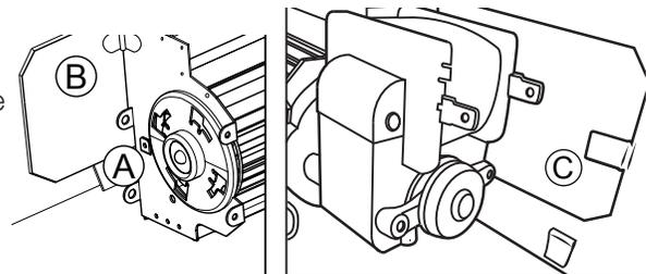
Drywall dust will penetrate into the blower bearings, causing irreparable damage. Care must be taken to prevent drywall dust from coming into contact with the blower or its compartment. Any damage resulting from this condition is not covered by the warranty policy.
