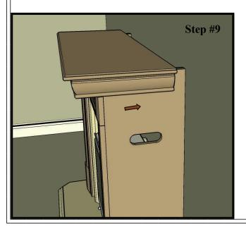
Insure that the firebox is centrally located on the hearth. Run gas line and venting, making sure that the hearth is not moved out of alignment. If installing the Tudor Vine, shaped or plain granite backpanels, or the cast plates, see page 3 of this guide for C channel installation.
