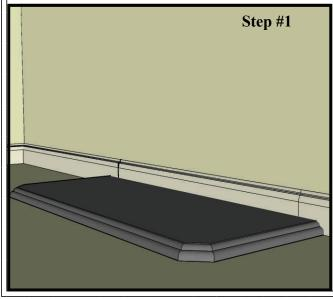
If there is a baseboard, carefully set the hearth into position and mark the base board where it must be cut. Make sure that the hearth is centered to the centre mark on the wall.
