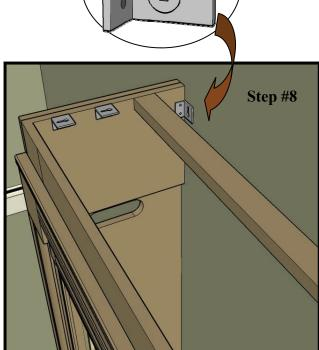
You may have to adjust the screw head in the wall plug to insure the mantel has a snug fit against the wall.
