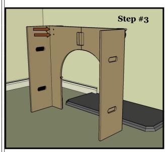
The two halves of the mantel can be connected together by inserting the bolts, washers, lock washers and nuts into the two wood cleats in the center of the back of the mantel.
