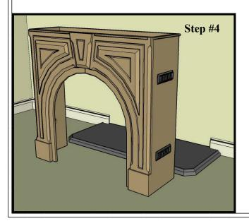
The center quoin can now be centrally positioned, and secured from behind with the 4 screws provided. Make sure that the screws are the correct length and do not protrude through the face of the quoin.
