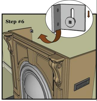
You may have to adjust the screw head in the wall plug to insure the mantel has a snug fit against the wall.
