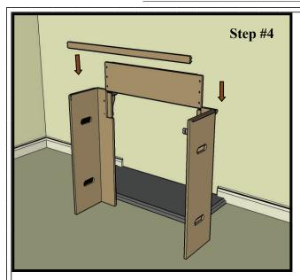
Once you have installed both corbels, carefully set the center beam and the mounting cleat into position. From the back of the mantel, secure the beam by using the 3 screws provided into the three holes on each side of the beam.
