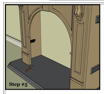
Place the mantel into final position on the wall, and mark the center of the top of the keyhole circle in the keyhole on each leg. Remove the mantel, and install the drywall plug centered on the mark you have just made. Set the screw into the wall plug so that the head is sticking out approximately 1/8" beyond the plug face. Reset the mantel into position, setting the screw head into the keyhole, and carefully allow the mantel to slid down into position.
