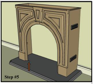
Insure that the firebox is centrally located on the hearth. Run gas line and venting, making sure that the hearth is not moved out of alignment.
