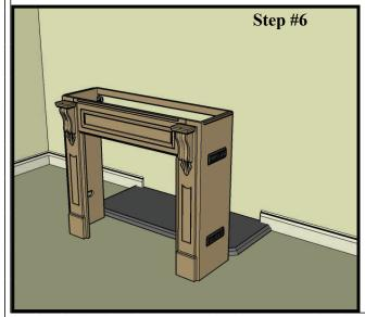
Install the 4 cast grills into the cutouts in the side of the mantel.
