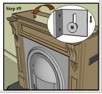
You may have to adjust the screw head in the wall plug to insure the mantel has a snug fit against the wall.
