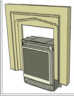
The backpanel can now be carefully lowered down the channel that is created. Insure that this is lowered evenly, and does not bind against the sides of the channel, as this may damage the inside corners of the backpanel.
