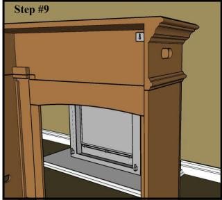
Check the fit and positioning of the mantel. Install the 4 cast grates into the holes on the sides of the mantel with the screws provided.
