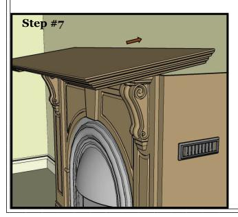
Set the mantel onto the hearth, and make a mark at the back of the inside opening of the mantel. Remove the mantel to the side. The 530 engine can now be installed, using this mark as the main reference point. Do a dry assembly of the Windsor front onto the 530 firebox, and set the front flat section of the Windsor plate on this line. It is this line that will determine the proper location of the firebox relative to the wall.
