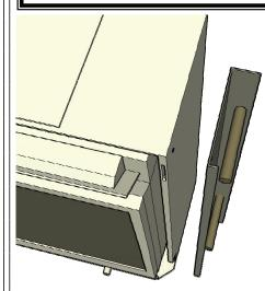
The 'C' channels are attached to the sides of the outer 530 box, and the backpanels are 'slid' down into the channels created. These backpanels are then held in place by the two threaded bolts from behind.
