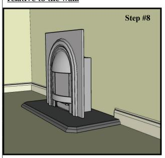
Place the mantel into final position on the wall, and mark the center of the top of the keyhole circle in the keyhole on each leg. Remove the mantel, and install the drywall plug centered on the mark you have just made. Set the screw into the wall plug so that the head is sticking out approximately 1/8" beyond the plug face. Reset the mantel into position, setting the screw head into the keyhole, and carefully allow the mantel to slid down into position.
