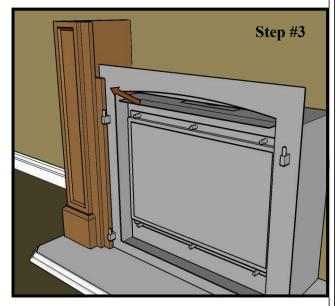
If installing the Barrington with one of the 530 and one of the backpanels, then you should again use the leg to locate the final resting point for the firebox and backpanel. Fit the C channels to the sides of the firebox [as shown on page 3], dry fit the backpanel to the firebox, and center this on the hearth. Carefully bring this to the back of the opening edge of the leg, and make a small pencil mark on the hearth indicating the final resting position.
