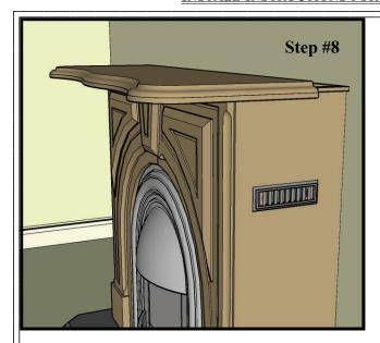
The shelf can now be slid into position, by carefully aligning it with the wooden side cleats, and gently pushing it backwards.
