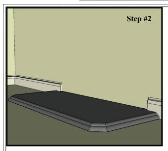
Use a fast set adhesive such as Kerakwik M to secure the hearth to the floor. Spread the adhesive across the bottom of the hearth where it comes in contact with the floor. Pick up the hearth on edge and lay the back edge against the wall. Slowly lower the leading edge and work the hearth back and forth to insure good adhesion. Wipe off excess adhesive with a damp cloth.
