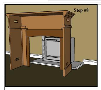
Once the two side slips are properly positioned and secured, you can now install the top slip.
