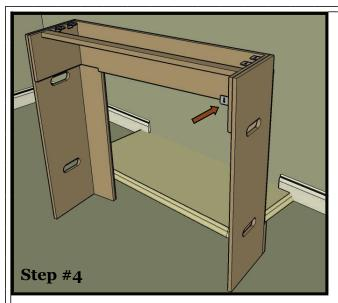
Screw the two key holed 'L' brackets to each side of the inside return of the leg, near the top. Make sure that the keyhole is located 'upside down'.
