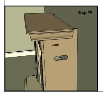
Insure that the firebox is centrally located on the hearth. Run gas line and venting, making sure that the hearth is not moved out of alignment. If installing the Tudor Vine, shaped or plain granite backpanels, or the cast plates, see page 3 of this guide for C channel installation.
