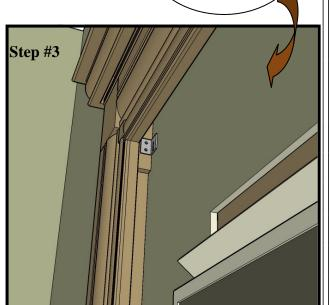
Carefully install the Tudor Vine as shown in on page 8. Reset the mantel into position by sliding the keyhole opening over the screw projecting from the wall plug, and then setting the mantel down into final position. You may have to adjust the screw head in the wall plug to insure the mantel has a snug fit against the wall.
