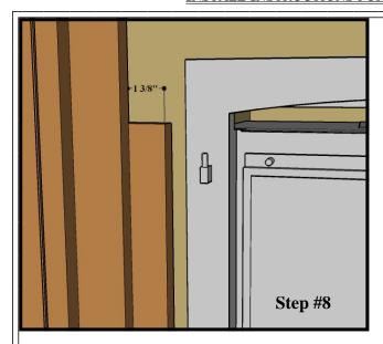
If you are installing the Barrington with the Fenderfire front, then you will need to install the wood slips onto the back of the opening of the mantel. Position a side slip so that there is 1 3/8" exposed on the front.
