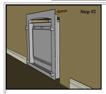
As the opening of the Barrington is the same as the Riversdale and the Kingston, this mantel can be installed with the rest of our backpanels, hearths and slips. In this case however, you must bring the front face of the slips 3" ahead of the drywall face. The example here shows the flat outer section of the Windsor face 3" ahead of the drywall.
