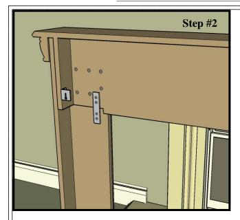
With the Tudor Vine front removed from the 530 firebox, put the assembled mantel into it's final position against the wall. While holding it carefully, make a mark on the wall at the top center point of the key hole in the wall mounting cleat.
