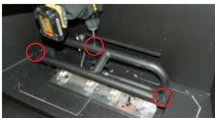
Diagram 2: Slide burner assembly to the right—then remove.
