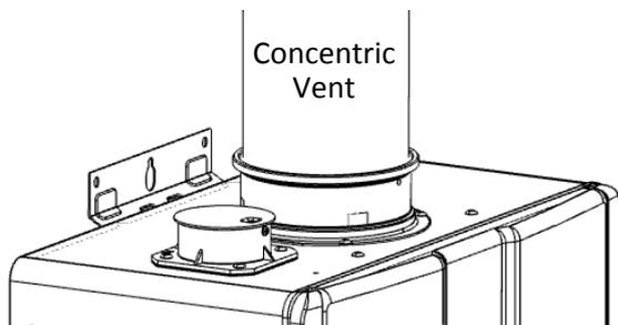
4. Secure the vent pipe to the concentric flue connection with the supplied screw.
