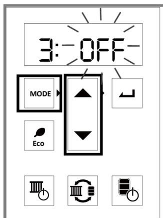
Press the **Mode** button three times. 3: OFF should appear on the display. Press the Up or Down arrows to select:
