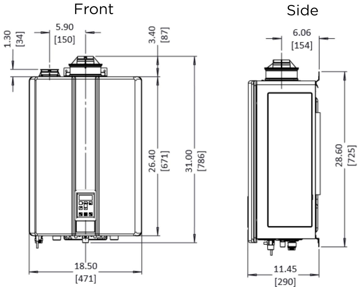
**Vent Connection:** 2 in. (51 mm) nominal PVC/Polypropylene or 3 in./5 in. Concentric
