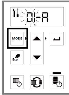
6. Press the ▲ (Up) or ▼ (Down) arrows until **A2-A** appears in the display. Then, press the **Select** button.
