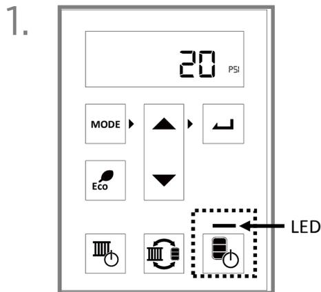
If the LED above the **Indirect Tank** button is not illuminated, press the **Indirect Tank** button.
