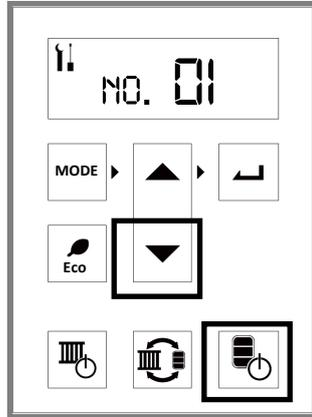
While continuing to hold the ▼ (Down) button, press and hold the **Indirect Tank** button (press and hold both buttons down at the same time).
