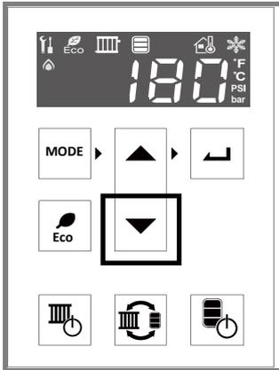
Press and hold the ▼ (Down) button for two seconds.
