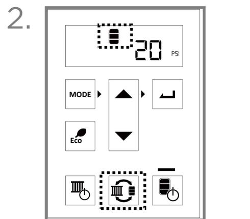
Press the **Switch Operation Mode** button until the **Indirect Tank** icon appears on the home screen.
