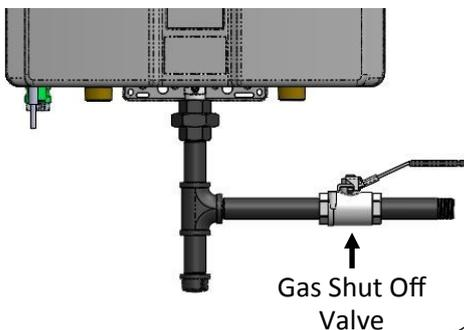
1. Check the type of gas and gas supply pressure before connecting the boiler. If the boiler is not of the gas type that the building is supplied with, converting the gas type of the boiler is necessary. A gas conversion kit is included with the boiler. Refer to section "14.4 Gas Conversion" in the Appendix for gas conversion instructions.
