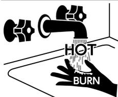
Water temperatures over 125° F (52° C) can cause severe burns or scalding resulting in death.
