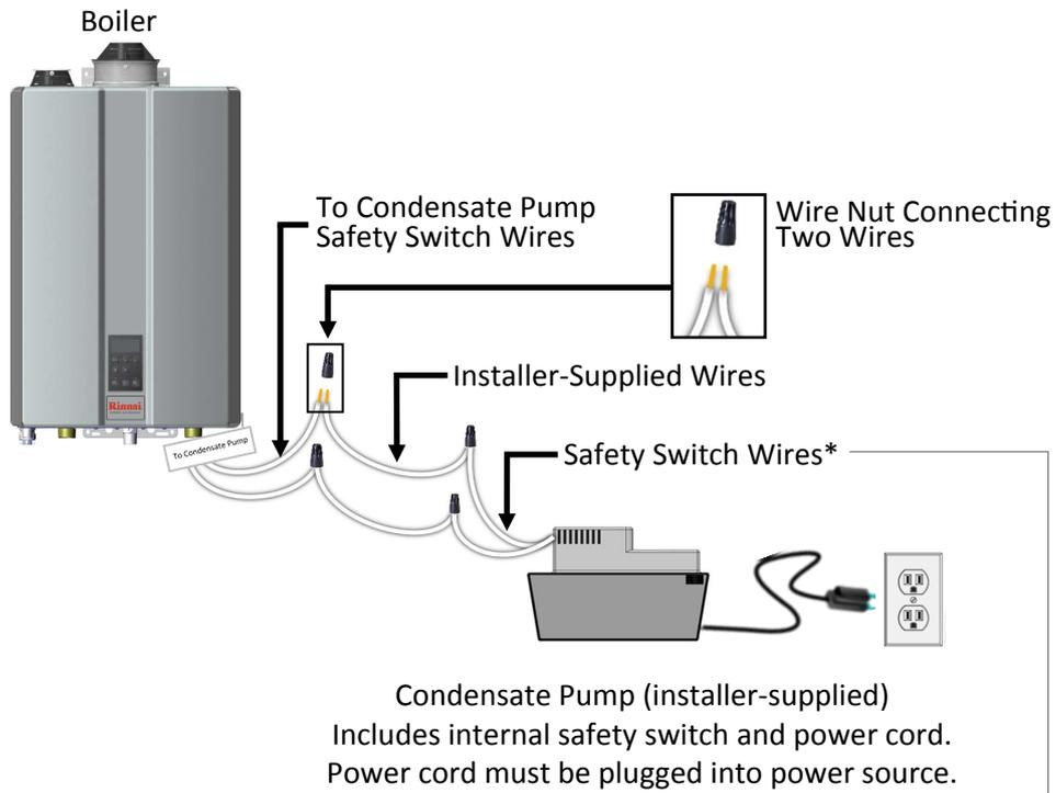
\* Safety switch wires connect to the NO and COM contacts on the safety switch.
