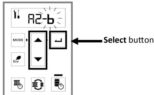
8. The boiler is now set to allow higher exhaust temperatures. To exit parameter settings and enter normal operation mode, press the **Mode** button.
