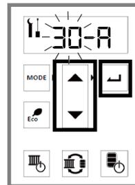
7. Press the ▲ (Up) or ▼ (Down) arrows to change the selection for the setting number (such as 30-A or 30-b).
