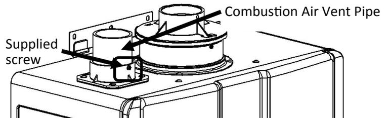
4. Place the vent screen or room air screen inside elbow and secure with the supplied screw. Use the room air screen for environments where room air is dusty.
