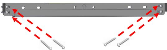
3. Insert the top bracket into the wall mounting bracket. Make sure the wall mounting bracket is attached to the wall and can hold the weight of the boiler before you fully let go.
