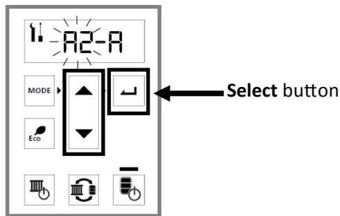
7. Press the ▲ (Up) or ▼ (Down) arrows until **A2-b** appears in the display. Then, press the **Select** button.
