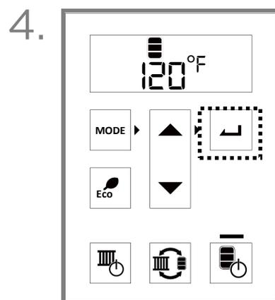
Press the **Select** button to confirm the temperature. The setpoint temperature displays for a few seconds and then returns to standby mode.
