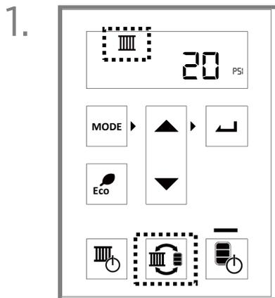
Press the **Switch Operation Mode** button until the **Central Heating Active** button appears on the home screen.
