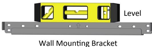
2. Use four screws to secure the wall mounting bracket to the wall (two screws on far left side and two screws on far right side).
