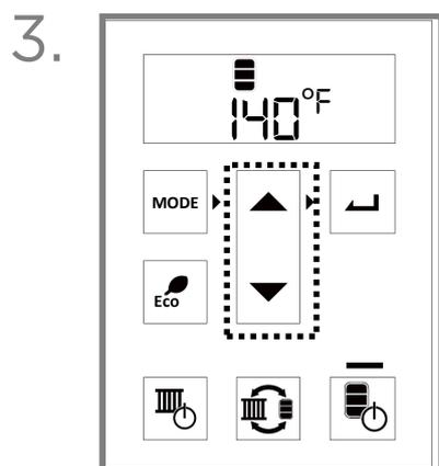
Adjust the temperature with the **Up** or **Down** arrows until the appropriate temperature is displayed.
