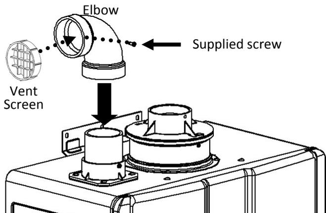
5. Install the exhaust vent pipe. Ensure it is properly seated. Secure the exhaust vent pipe to the exhaust adapter ring with the supplied screw.
