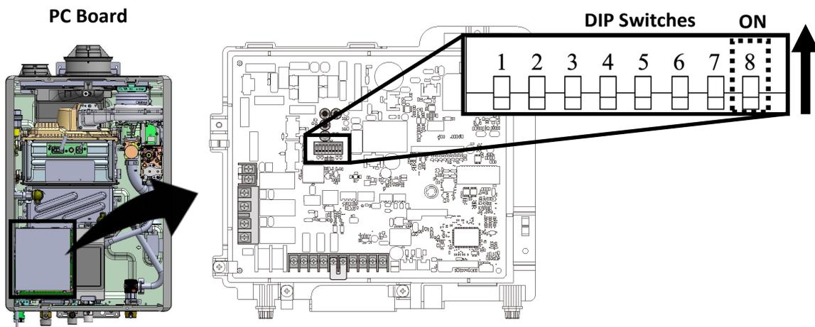
4. On the PC Board, press and hold the red button for five seconds
