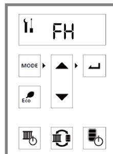
6. To enter back into normal operation, press the right-side, black button. The controller now displays normal operation mode.
