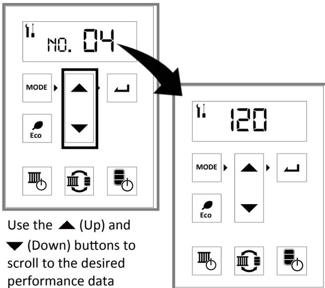
Use the ▲ (Up) and ▼ (Down) buttons to scroll to the desired performance data number described in the **Performance Data Table** in this section.
