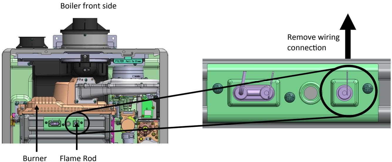
**WARNING** Do not touch the inside of the wiring connection while it is disconnected.
