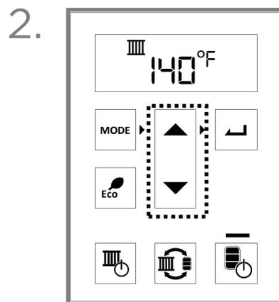
Adjust the temperature with the **Up** or **Down** arrows until the appropriate temperature is displayed.
