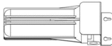
Filters and reduces the amount of scale entering the boiler allowing for greater boiler longevity.
