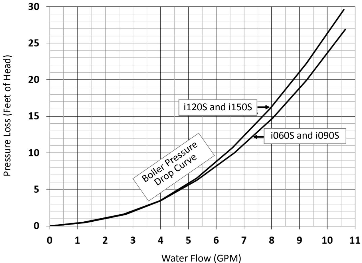
Below are options for the primary pump circulating across the boiler. No additional pressure drop is accounted for through the system piping or system components. Recommended circulation pumps are listed below. The maximum amperage permitted is 2 Amps.
