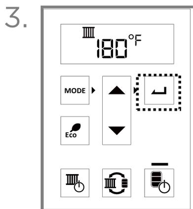
Press the **Select** button to confirm the temperature.
