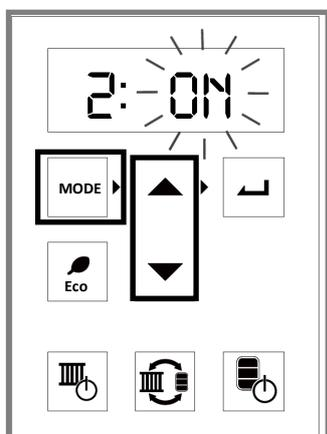
Press the **Mode** button twice. **2:ON** should appear on the display. Press the **Up** or **Down** arrows to select ON or OFF.
