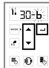
8. To exit parameter settings and enter normal operation mode, press either the red button on the PC Board or the **Mode** button on the controller.
