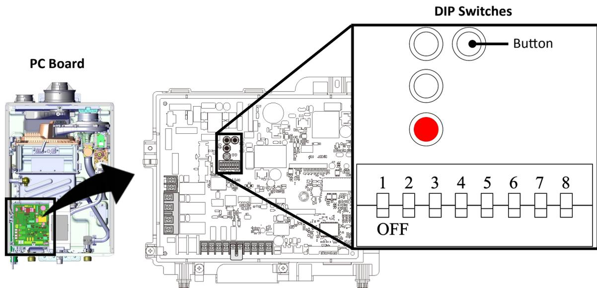
4. The controller displays **FL** (the boiler is now in forced low fire condition).
